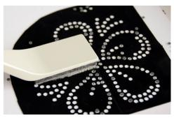
**step 4.** Place the glitter iron-on transfer material onto a standard ScanNCut mat and load into the machine. Select pattern(s) and cut.
