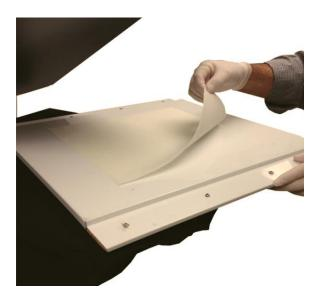
9. Press the garment using a hot press at 356°F for 35 seconds with 80psi to dry (cure) the pretreat. Cover the pretreated area with a Teflon sheet or use a Teflon cover (bra) on the upper heat element and lower platen base. This will give you the best results for both pretreat and ink curing.
