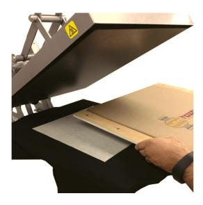
7. Press the garment using the Pretreat Paper Platen on the hot press for 35 seconds at 60 to 65psi. This is a cold press and is designed to transfer over the pretreat solution form the paper with no heat. On this application the heat is not a factor as the Pretreat Platen pad obstructs the heating element.
