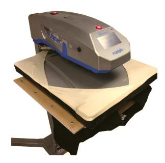
8. After pressing remove the paper from the bottom side of the Pretreat Paper Platen. The paper has a onetime use only, and must be discarded after use.
