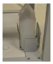
3. Place the waste tube in the tank, (remember to cut the tube in accordance with the tank).
