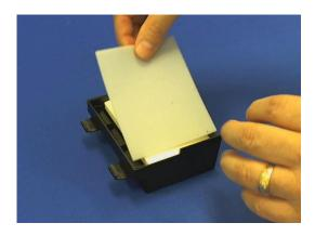
3. Install the assembled flushing plate into the machine.
