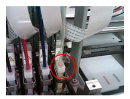
16. Place the cable (silver side up) into the black tabs from step 10, and lock into place by pushing the tab away from you (towards the capacitor).
