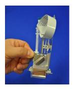
12. Mount the print head on the printer; fit the V-shaped groove to the positioning pin.
