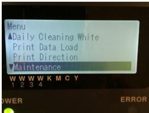
3. Select [ Maintenance Parts Exchange ] and press OK Button. The Platen will be loaded and the Wipers will be moved to the cleaning position. Follow the message and turn off the printer.
