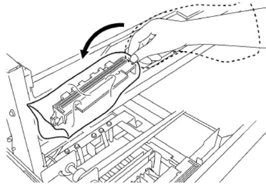
8. Remove the wrapped Wiper Cleaner carefully, not to drop waste ink and dispose of in accordance with local regulations.
