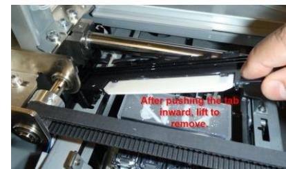
6. Move the Wiper Cleaner slightly to the left (1-2 mm) to release the claw in the left. Pay attention not to tilt the Wiper Cleaner or the waste ink may drop. Keep flat and move slowly.
