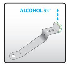
**Gently slide** the tool across the **encoder strip**, remembering to move the carriage to get the other side of the strip.
