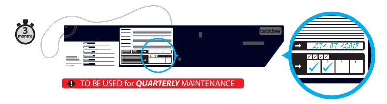
This **Maintenance Cartridge for CMYK** should be used to perform the **CTC** every **three months**. It is the only way **to clean** easily all the little **color tubes inside** the Maintenance station and keep a good suction of the pump to clean PrintHeads. > It is also a consumable like the MNT Cartridge for White. Mark the date or check the 5L bottles.
