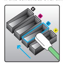
**Moisten** a swab as done for the wiper blade cleaning, and **swab the edges** and the **inside** of the **rubber caps**.
