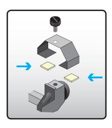
The **Carriage** contains **2 brackets** on the front edge that hold **4 felt pads** onto Velcro inserts.
