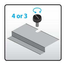
**Loosen** the four (or three, depending of model) black thumb **screws** (do not remove them completely) of the encoder cover, and remove the cover.
