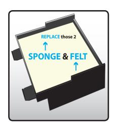
Insert the **felt** into the **flushing plate**.
