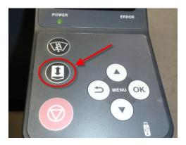
15. Press the Up/Down button to select "initial" cleaning mode, and then press the okay button.
