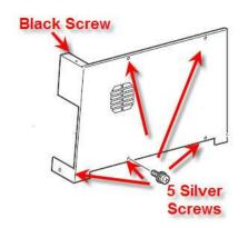
3. Remove the Four Silver Phillips Screws from the side cover and lift the cover from the machine.
