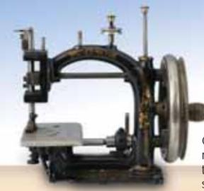
Chain-stitch sewing machine for the production of straw hats
