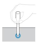
When using the eyelet punch, place thick paper or some other protective sheet under the fabric before punching the hole in the fabric.
