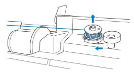
4 Hold the thread end with your left hand, and wind off the thread clockwise with your right hand as shown below.
