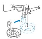
Tighten the screw with the included screwdriver.
