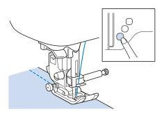
Press the (1) (Thread cutter button) to trim the upper and lower threads.
