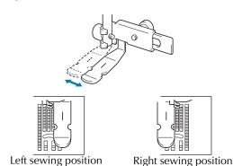
6 Change the needle position so that the needle does not touch the presser foot.
