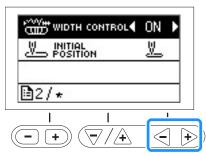
→ The machine is now set so that the stitch width can be controlled with the sewing speed controller.
