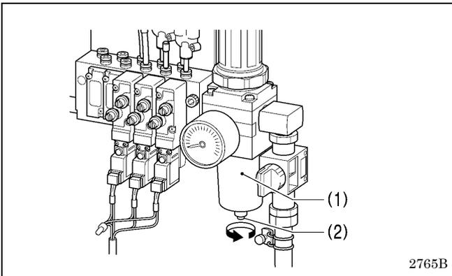
1. If water collects in the bottle of the regulator (1), turn the drain cock (2) in the direction of the arrow to drain the water.
