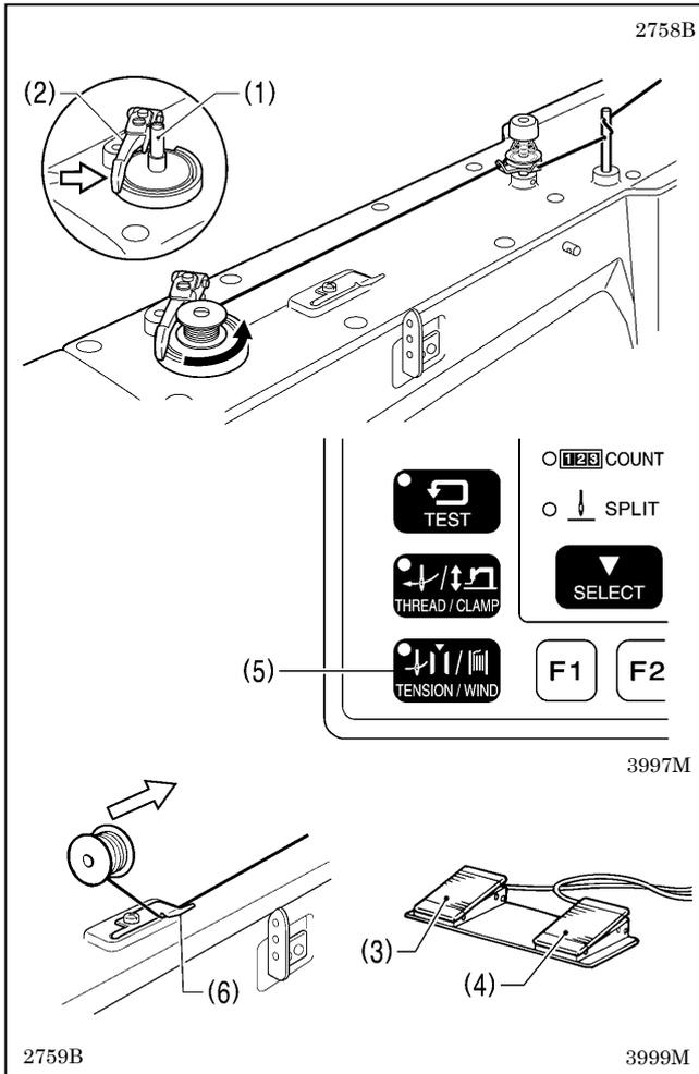
1. Place the bobbin onto the bobbin winder shaft (1).
