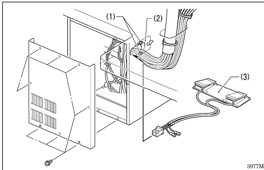
1. Remove the cover of the control box.
