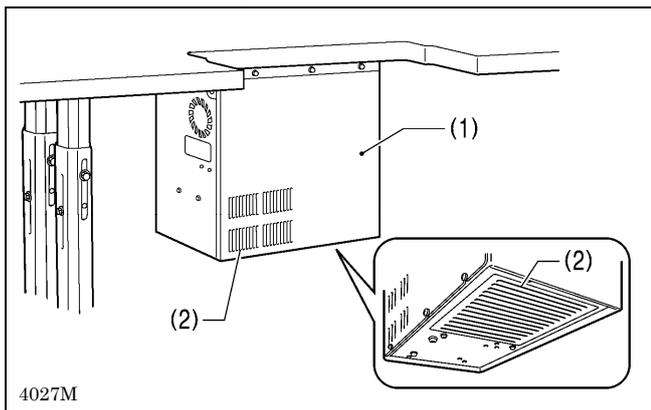
Use a vacuum cleaner to clean the filter in the air inlet ports (2) of the control box (1) at least once a month.
