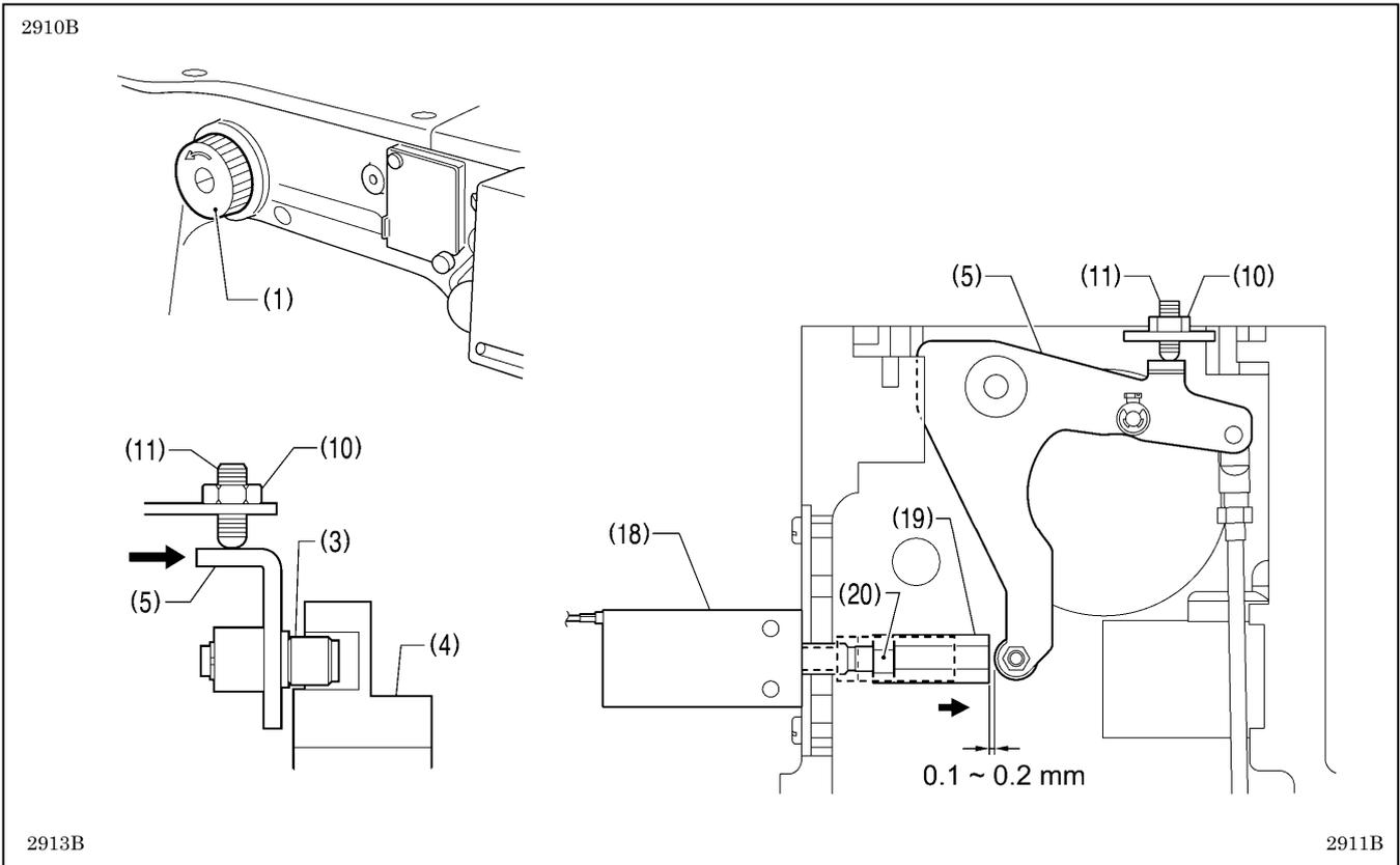
7. Turn the pulley (1) by hand to move the needle bar to its lowest position.
