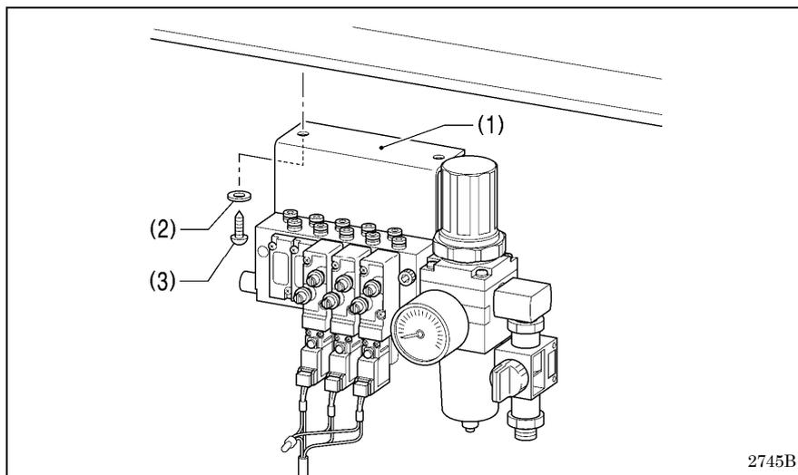
Install underneath the work table. (Refer to "3. Table processing diagram" for the installation positions.)
