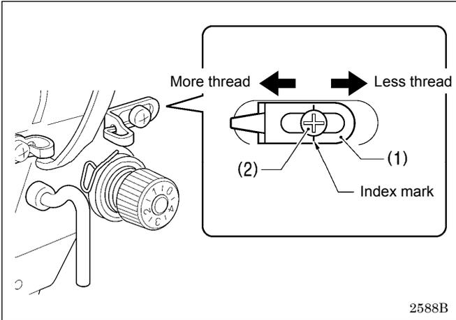
The standard position of arm thread guide R (1) is when the screw (2) is aligned with the index mark. Loosen the screw (2) and move arm thread guide R (1) to adjust.
