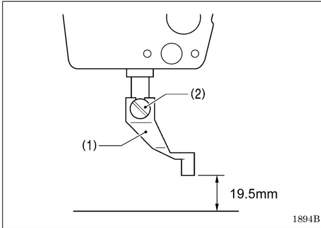
Install the intermittent presser foot (1) with the screw (2) so that the distance from the bottom of the intermittent presser foot to the top of the needle plate is 19.5 mm when the sewing machine is stopped and the intermittent presser foot (1) is raised.
