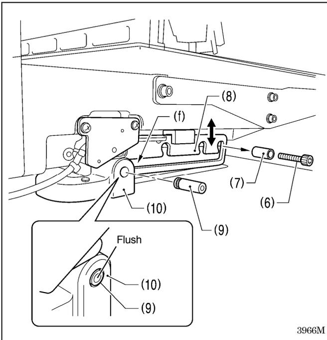
2. After placing the machine head onto the table, remove the bolt (6) and the spacer (7).
