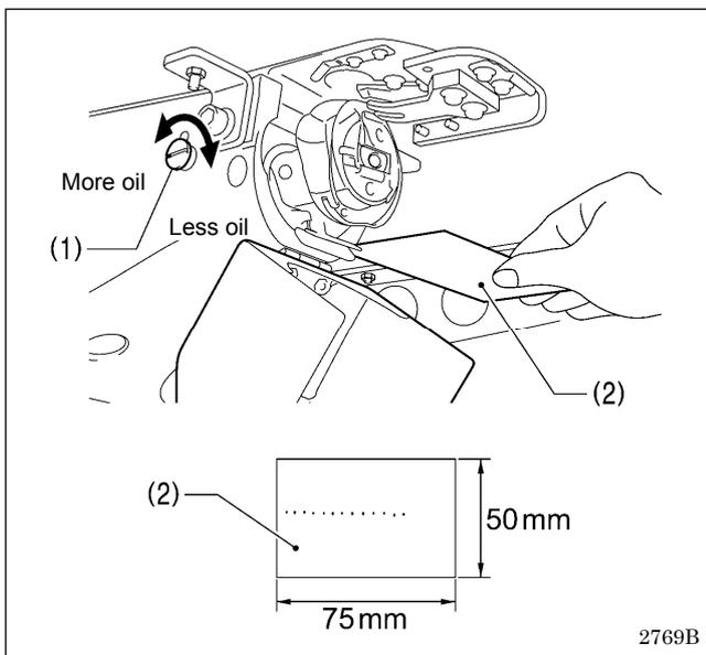
Turn the adjusting screw (1) to adjust the lubrication amount.
