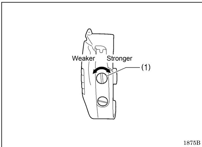
Adjust the lower thread tension by turning the adjusting screw (1).
