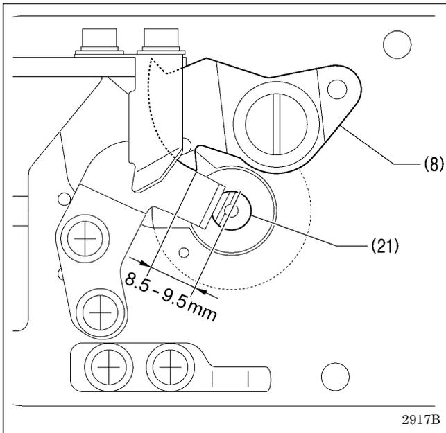
16. Check that there is a gap of about 8.5 – 9.5 mm between the tip of the movable knife (8) and the center of the hole in the needle hole plate (21) when there is still play between the parts.
