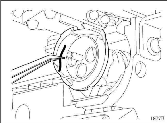
Remove the bobbin case, and then remove the thread scraps and lint from around the shuttle. Also wipe the bobbin to remove oil.
