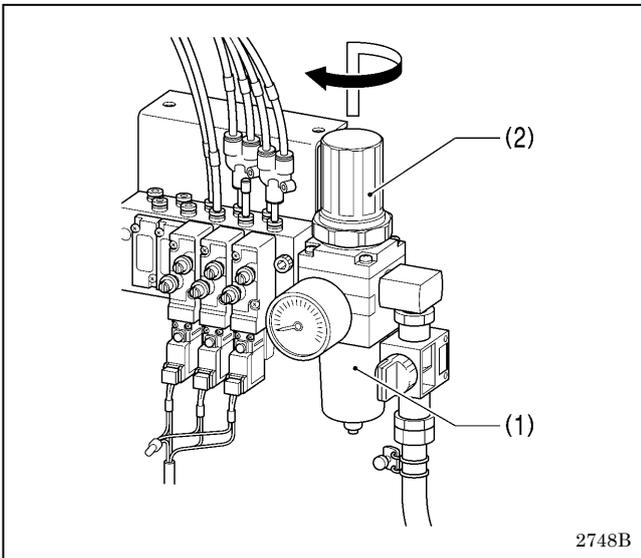
Lift up the handle (2) of the regulator (1) and then turn it to adjust the air pressure to 0.5 MPa. After adjustment is complete, push the handle (2) downward to lock it.
