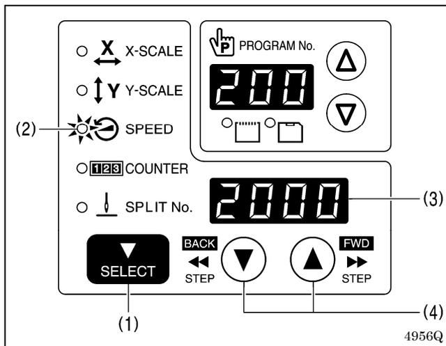
The sewing speed is set to 2000 (sti/min) at the time of shipment from the factory.
