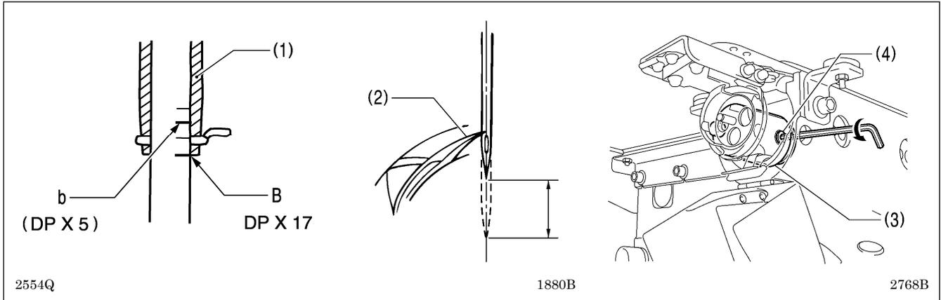
Turn the machine pulley to raise the needle bar from the lowest position until the lowest reference line on the needle bar (reference line B) is aligned with the lower edge of the needle bar bush (1), and then adjust the two set screws (4) of the rotary hook joint (3) so that the rotary hook tip (2) is aligned with the center of the needle.
