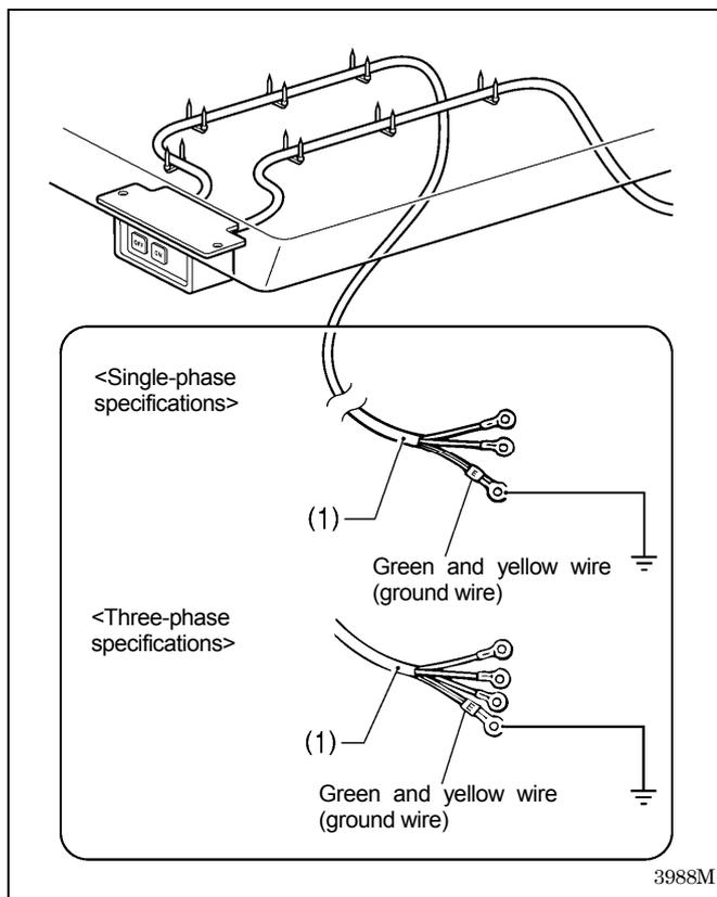
1. Attach an appropriate plug to the power cord (1). (The green and yellow wire is the ground wire.)
