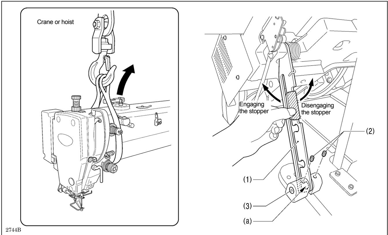
1. Tilt back the machine head, and then secure the support lever (1) at stopper position (a).
