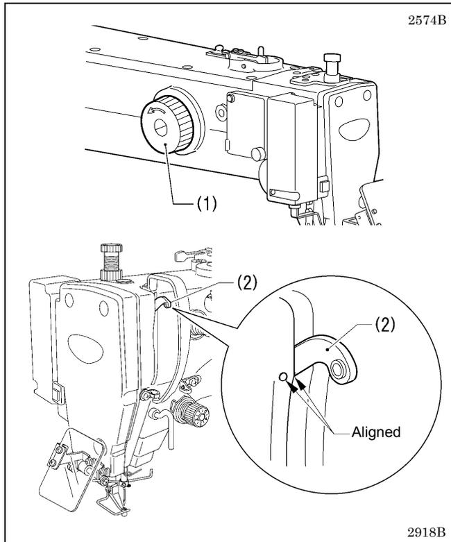
Before starting home position detection, check that the needle bar is at the needle up stop position.
