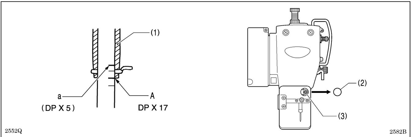
Turn the machine pulley to move the needle bar to the lowest position. Then remove the rubber plug (2), loosen the screw (3) and then move the needle bar up or down to adjust so that the second reference line from the bottom of the needle bar (reference line A) is aligned with the lower edge of the needle bar bush (1).
