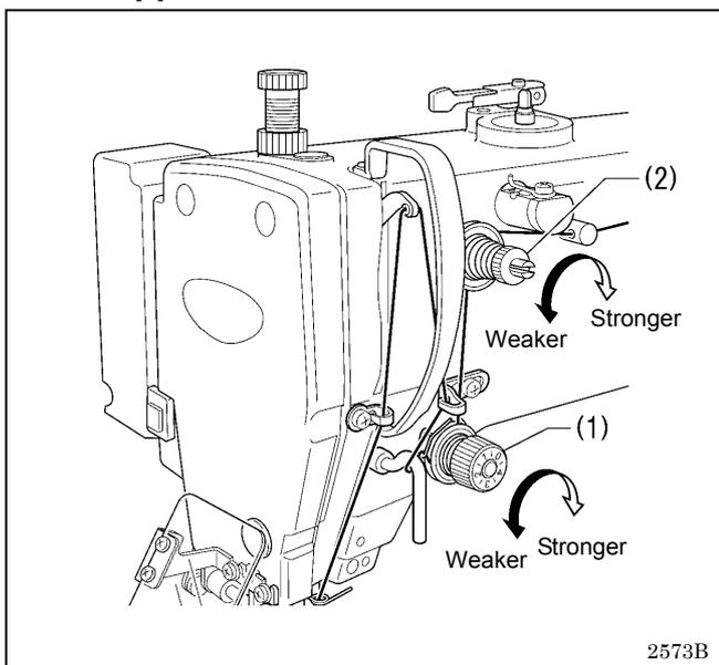
1. Turn the tension nut (1) (main tension) to adjust the tension as appropriate for the material being sewn.
