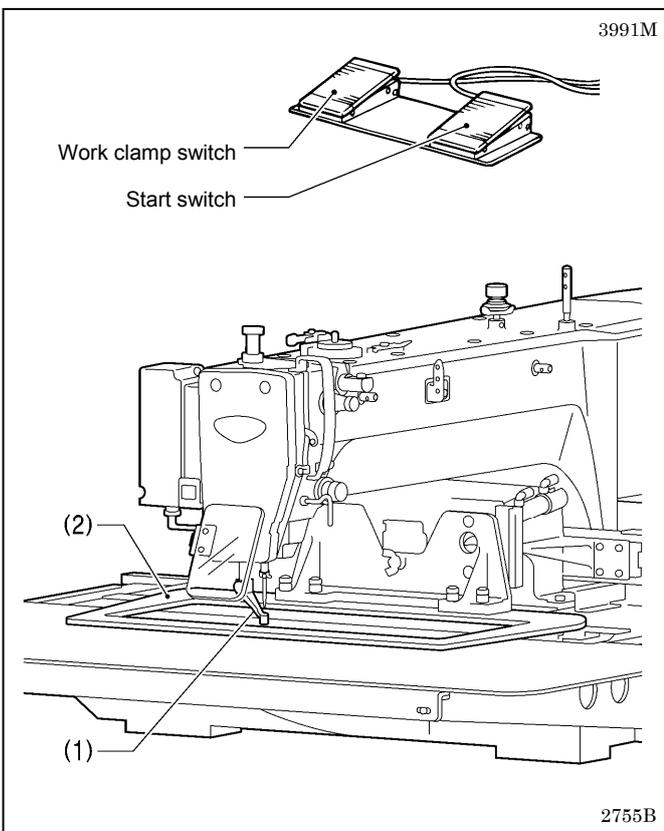
When the work clamp switch (left side) is depressed, the intermittent presser foot (1) and the work clamp (2) are lowered, and when the start switch (right side) is then depressed, the sewing machine starts operating.
