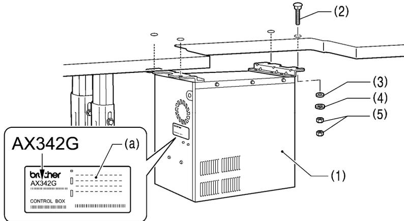
Before installing the control box (1), check that the model plate (a) on the control box (1) is "AX342G" to indicate that it is an RX-control box for BAS-342G sewing machines.
