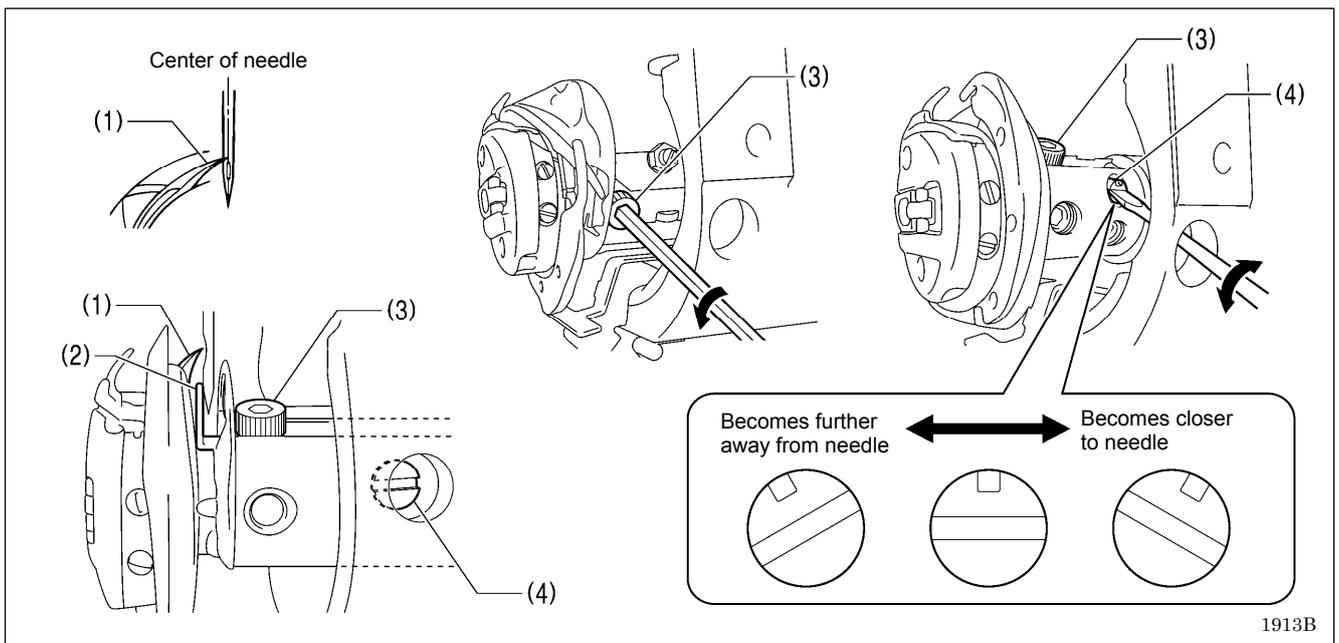
Turn the machine pulley to align the tip of the rotary hook (1) with the center of the needle, and then loosen the bolt (3) and turn the needle guard adjusting shaft (4) to adjust so that the driver needle guard (2) is touching the needle.
