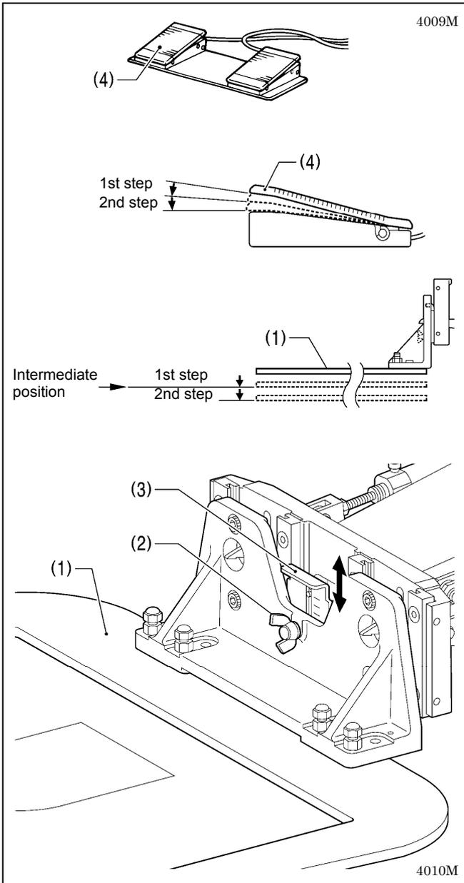
When these settings are made, the work clamp (1) can be lowered in two steps.
