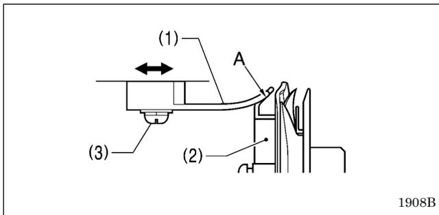
Loosen the two screws (3) to adjust so that the tip of the hook stopper (1) does not protrude past edge A of the inner rotary hook (2).
