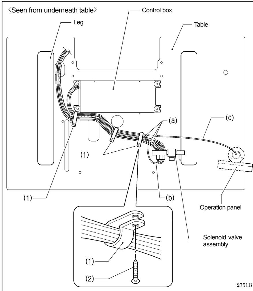
Secure the three air tubes (a), the solenoid valve assembly cord (b) and the operation panel cord (c) together underneath the table with the three cord holders (1).
