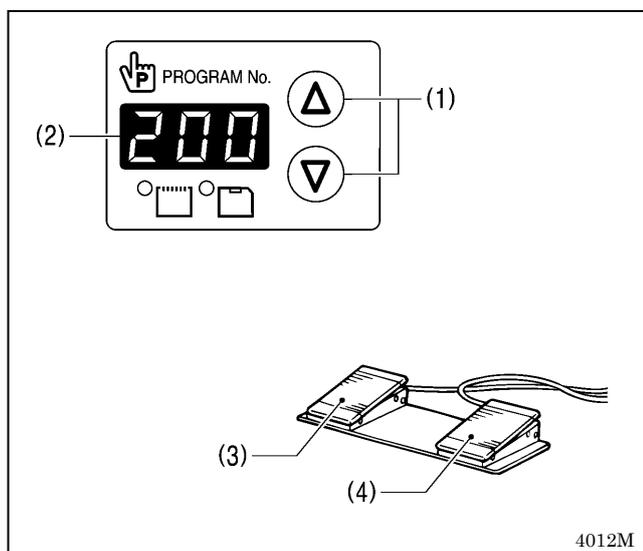
1. Press the  $\Delta$  or  $\nabla$  key (1) to select the program number that is loaded into the internal memory.
