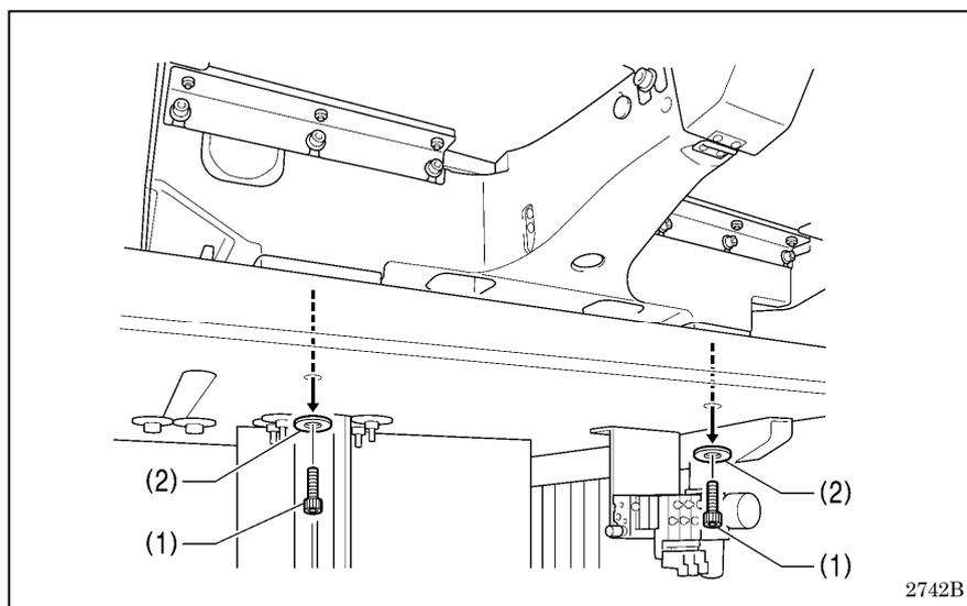
If the sewing machine was already installed to the table when it was delivered, remove the two machine head fixing bolts (1) and the two plain washers (2).
