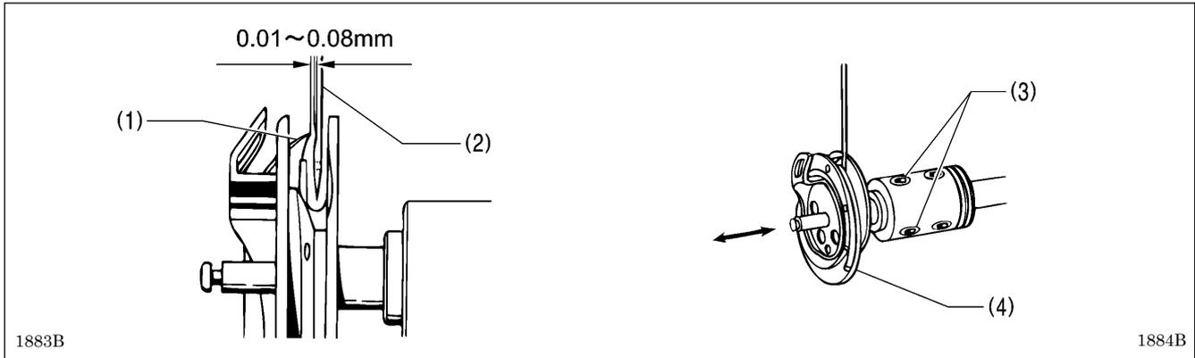
Turn the machine pulley to align the rotary hook tip (1) with the center of the needle (2), and then loosen the two set screws (3) and move the rotary hook (4) forward or back to adjust so that the clearance between the needle (2) and the rotary hook tip (1) is 0.01 – 0.08 mm.
