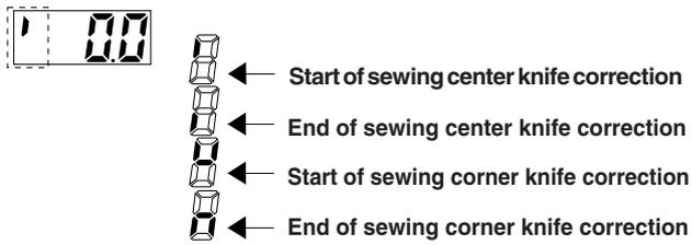
The diagram shows a digital display with '00' and a dashed box around it. To the right are four vertical icons representing sewing knives. Arrows point to each icon with labels: 'Start of sewing center knife correction', 'End of sewing center knife correction', 'Start of sewing corner knife correction', and 'End of sewing corner knife correction'. | Setting for the center and corner knives |
