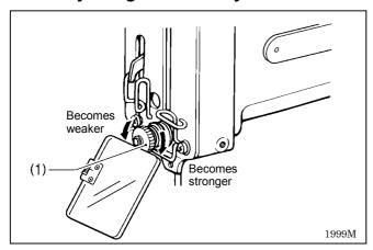
The auxiliary tension is adjusted by turning the tension nut (1).
