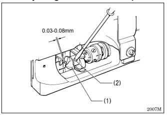
Adjust so that the clearance between the needle and the tip of the looper (1) is 0.03-0.08 mm when the needle bar rises from its lowest position until the tip of the looper (1) is aligned with the center of the needle.
