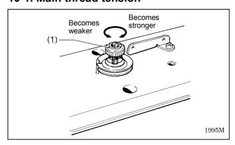
The main thread tension is adjusted by turning the tension nut (1).
