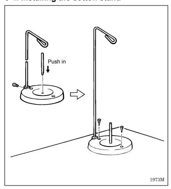
Assmble the cotton stand as shown in the illustration, and then install it to the far right corner of the table with the two wood screws.
