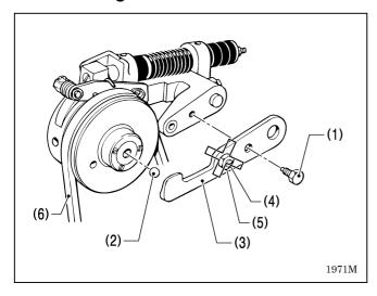
Loosen the screw (1), and then remove the ball presser plate (3) while being careful not to drop the bearing ball (2).
