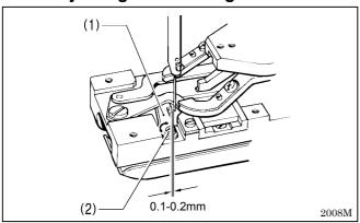
Adjust the clearance between the needle and the needle guard (1) to 0.1-0.2 mm.
