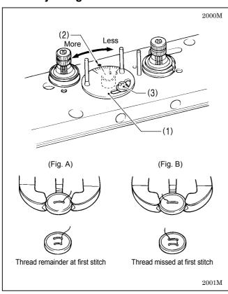
The standard position for the rotor (1) at the sewing machine stopping position is the position where the <1.5> scale indicator should be aligned with the index mark (2).
