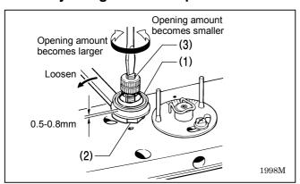
Adjust so that the tension disc presser (1) opens by 0.5-0.8 mm when the sewing machine starts (when the machine pulley is turned by hand).
