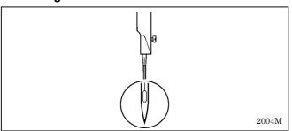
If the needle tip is bent or broken, replace the needle.
