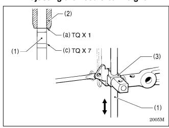
Adjust so that reference line (a) on the needle bar (1) is aligned with the bottom edge of needle bar bush D (2) when the needle bar (1) is at its lowest position.
