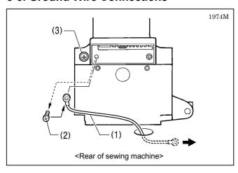
Connect the ground wire to the sewing machine head and motor. (Use the correct type of ground wire.)
