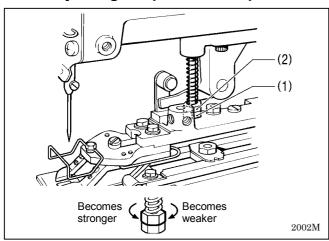
Adjust the pressure to be as weak as possible so that the material does not slip when it is pulled gently.
