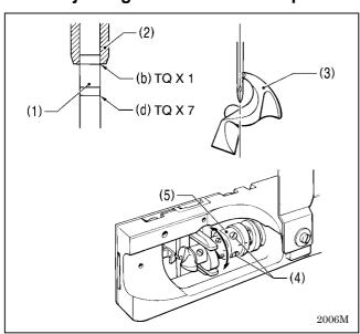
Adjust so that the tip of the looper (3) is aligned with the center of the needle when the needle bar (1) rises from its lowest position until reference line (b) of the needle bar (1) is aligned with the bottom edge of needle bar bush D (2).
