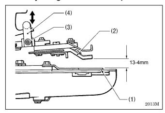
Adjust the distance from the top of the feed plate (1) to the edge of the button clamp (2) to 13-14 mm.
