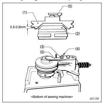
At the sewing machine stopping position, adjust the clearance between the machine pulley (1) and the clutch plate (2) to 0.5-0.8 mm.
