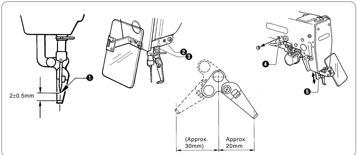
1. Loosen the set screw **2** and move the wiper arm support **3** up or down to adjust so that the clearance between the top of the thread wiper and the needle point **1** is  $2 \pm 0.5$  mm when the thread wiper is aligned with the center of the needle.
