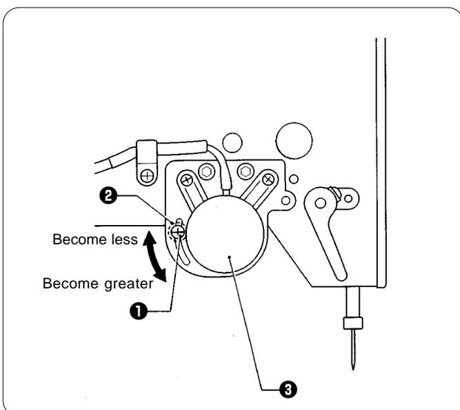
Loosen the screw ❶ and move the stopper (3.57 nut) ❷ to adjust the operating angle of the thread take-up solenoid ❸.
