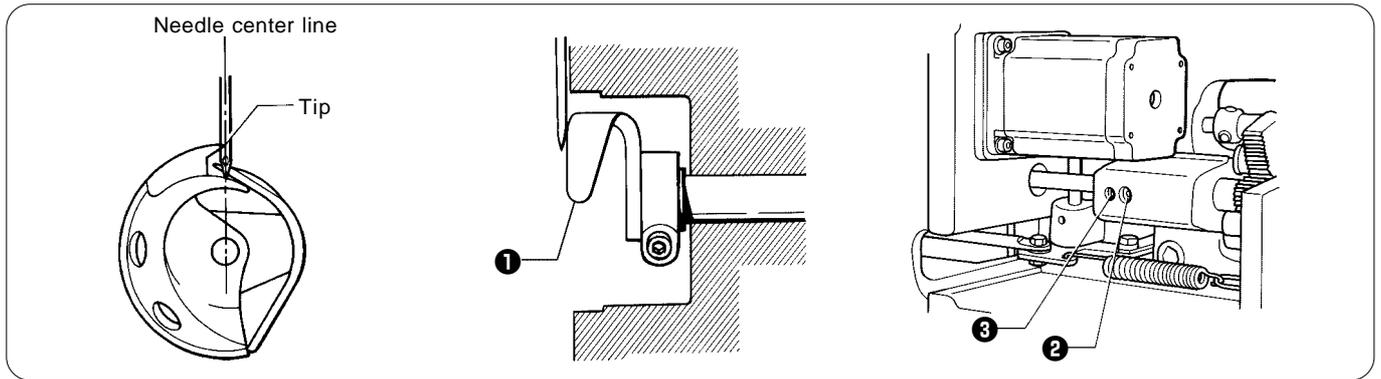
Turn the machine pulley to align the tip of the rotary hook with the needle center line. Then loosen the set screw **2** and turn the eccentric shaft **3** to adjust so that the driver needle guard **1** contacts the needle. If the needle contact pressure is too great, skipped stitches may occur. On the other hand, if the driver needle guard **1** is not touching the needle, the tip of the inner rotary hook will obstruct the needle, resulting in an excessively high amount of friction.
