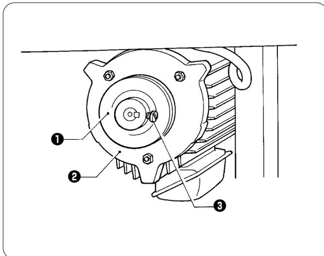
Place the motor pulley **1** onto the shaft of the motor **2** so that the key groove is aligned, and then tighten the set screw **3** so that the center of the V groove in the motor pulley **1** is aligned as closely as possible with the center of the belt hole in the power table.
