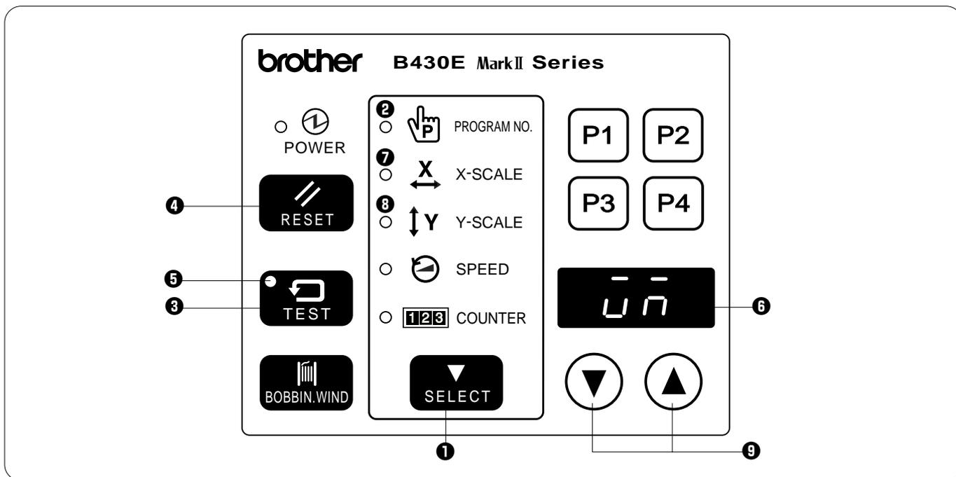
1. Select the program number, and then press the start switch once to move the feed mechanism to the sewing start position.
