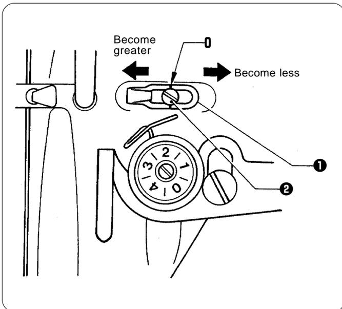
The standard position of arm thread guide R ❶ is when the screw ❷ is aligned with mark 0.
