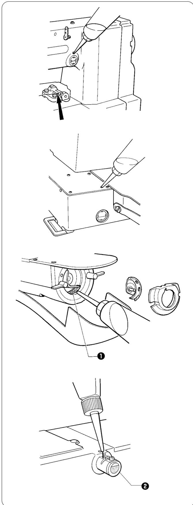
1. Fill the arm-side oil tank with oil.
