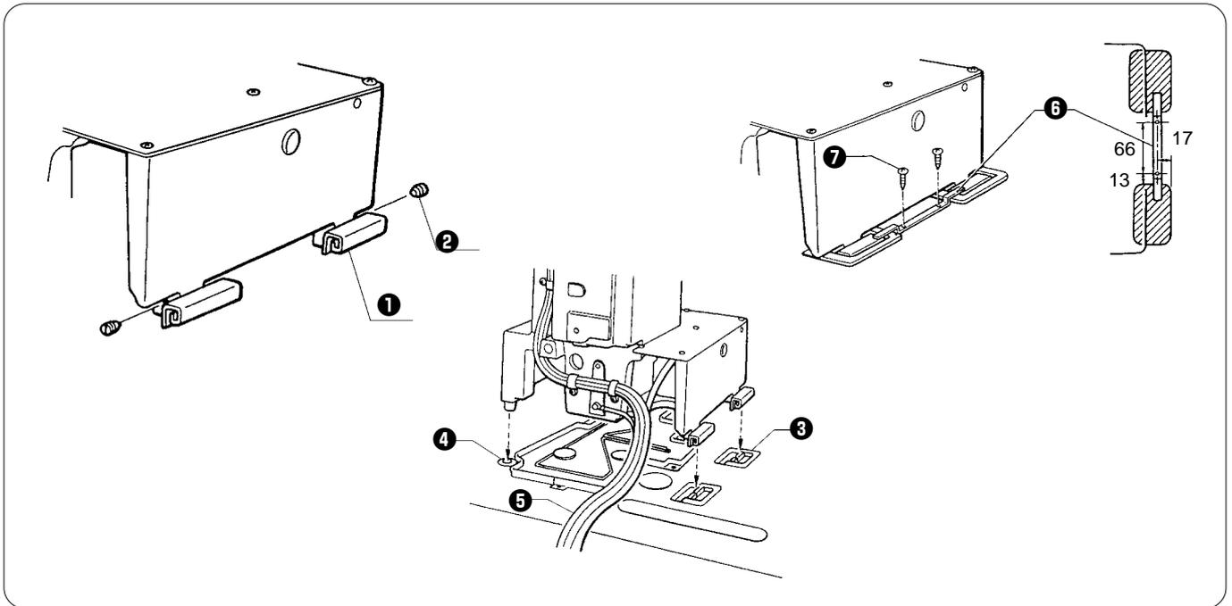
1. Insert the head hinges **1** into the machine head so that they are parallel, and then secure them with the two set screws **2**.
