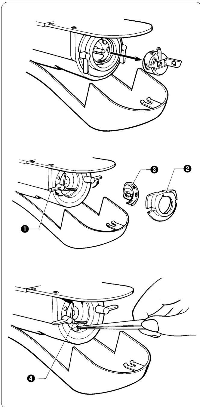
1. Pull the shuttle race cover toward you to open it, and then remove the bobbin case.
