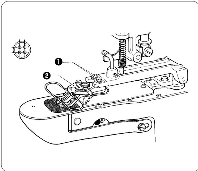
1. Loosen the two hexagonal bolts ① and adjust the button holder body ② by moving it.
