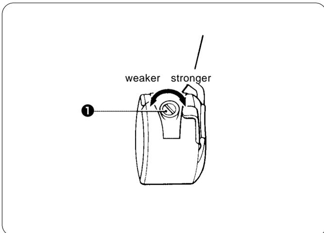
Adjust the thread tension to the weakest possible tension by turning the thread tension nut **1** until the bobbin case will not drop by its own weight while the thread end coming out of the bobbin case is held.
