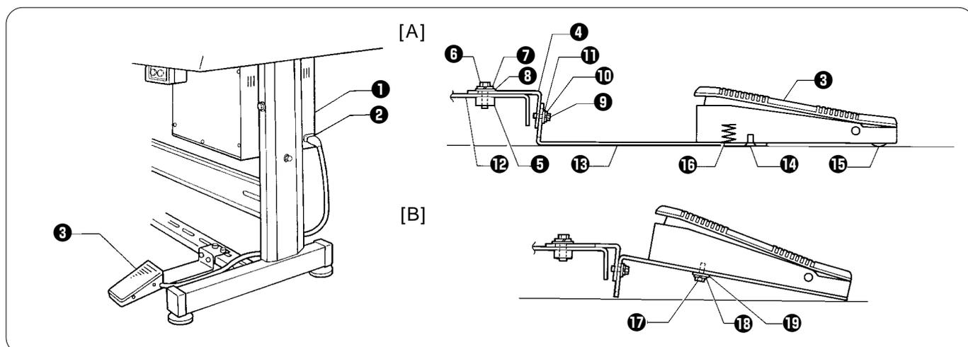
1. Insert the connector of the foot switch **3** into the connector **2** of the control box **1**.
