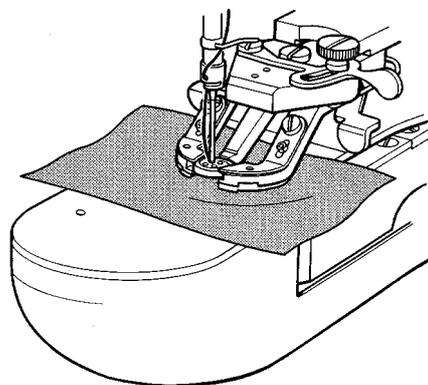
5. Once sewing is completed and the thread has been trimmed, the button clamp will rise.
