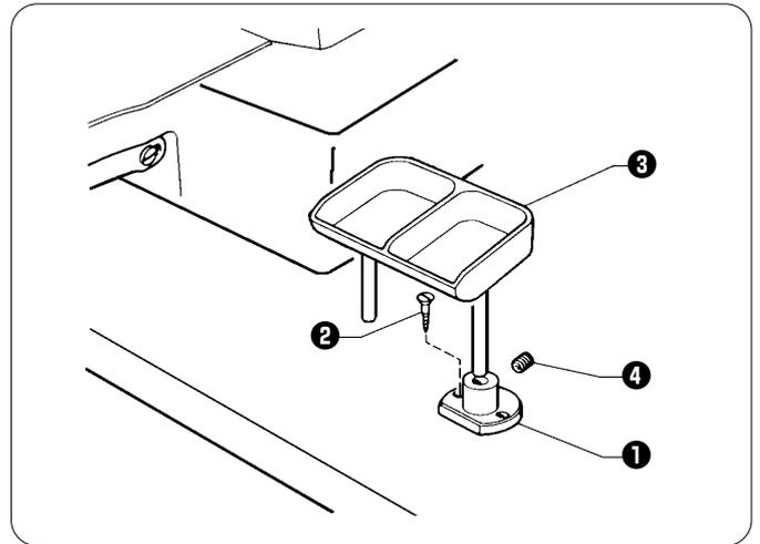
1. Install the button tray holder **1** with the two flat wood screws **2** at a place convenient for operation.
