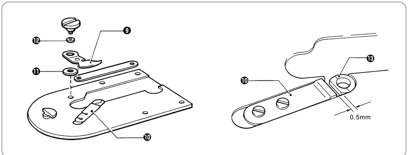
4. Remove the movable knife **9** and replace it with a new one. At this time, check that the movable knife **9** and the fixed knife **10** cut the thread cleanly. If necessary, adjust by using the appropriate movable knife washer **11** (supplied as accessories).
