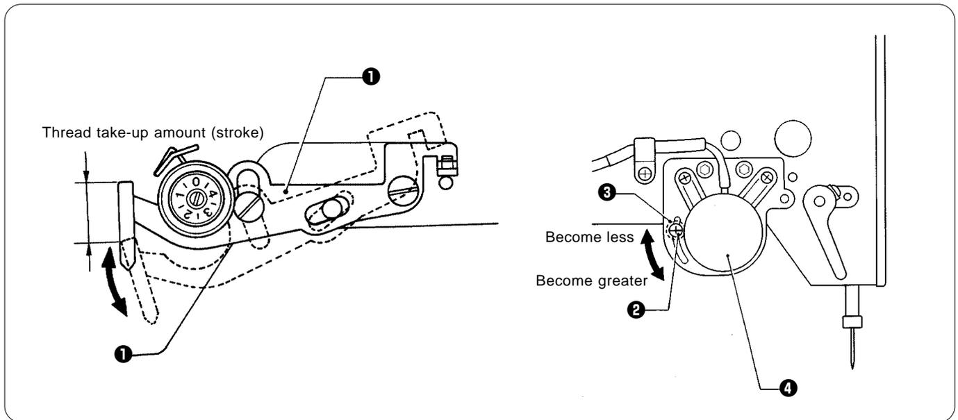
At the time of shipment from the factory, the thread take-up amount (stroke) of the thread take-up lever **1** is set to the standard setting of 5 mm. You may need to adjust this setting depending on the sewing conditions to prevent the thread from pulling out at the sewing start.
