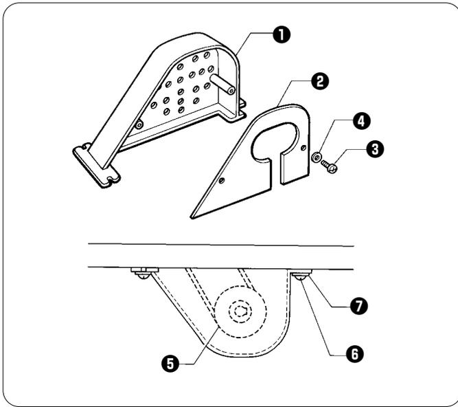
1. Install the motor cover **1** to the motor back cover **2** with the screws **3** and the flat washers **4**.
