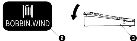
5. The bobbin presser **1** will automatically return to its original position after a set amount of thread (80 - 90% of the bobbin capacity ) has been wound on.
