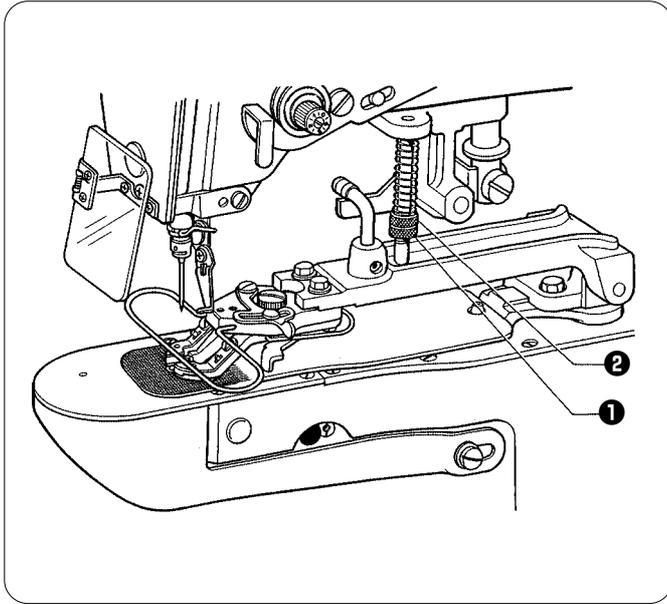
Loosen the adjusting nut ① and turn the adjusting nut ② to the point where it is just tight enough that the material will not slip out of place when it is slightly pulled (keep pressure as slight as possible).
