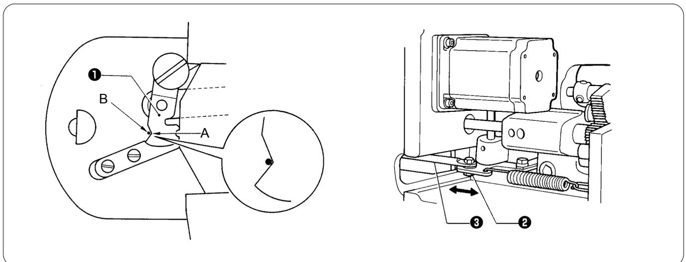
Loosen the nut **2** and move the connecting rod lever **3** to the left or right to adjust so that the V section A is aligned with the index mark B on the needle plate when the sewing machine is in the stopped position and the movable knife **1** is moved toward the index mark.
