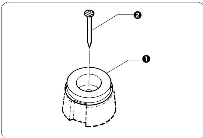
Place the two cushions **1** into the holes in the work table so that the notches are aligned with the tabs in the oil pan, and secure them in place with the nails **2**.
