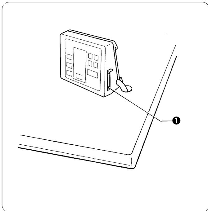
The operation panel DIP switches ❶ are used to change functions which might need to be changed depending on the sewing conditions.
