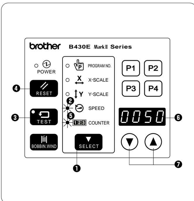
1. Press the SELECT switch **1** until the SPEED indicator **2** illuminates.
