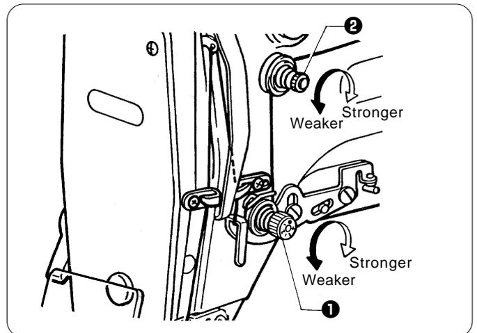
Turn the tension nut **1** (main tension) to adjust the tension as appropriate for the material being sewn. Furthermore, turn the thread nut **2** (sub-tension) to adjust the remaining length of upper thread to 35 - 40 mm when the thread take-up lever is not used.
