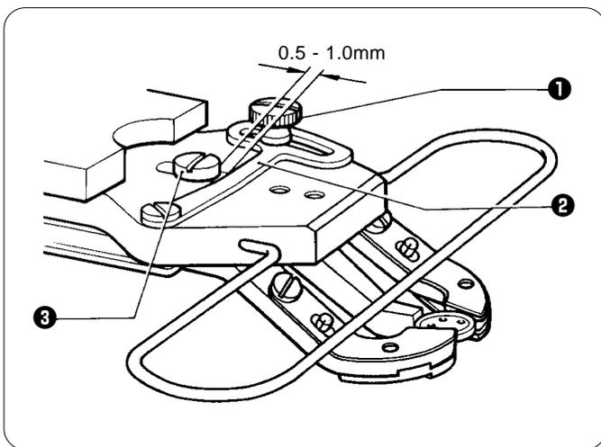
1. Insert the button in the button holder. Confirm that the button is securely held by the holder.
