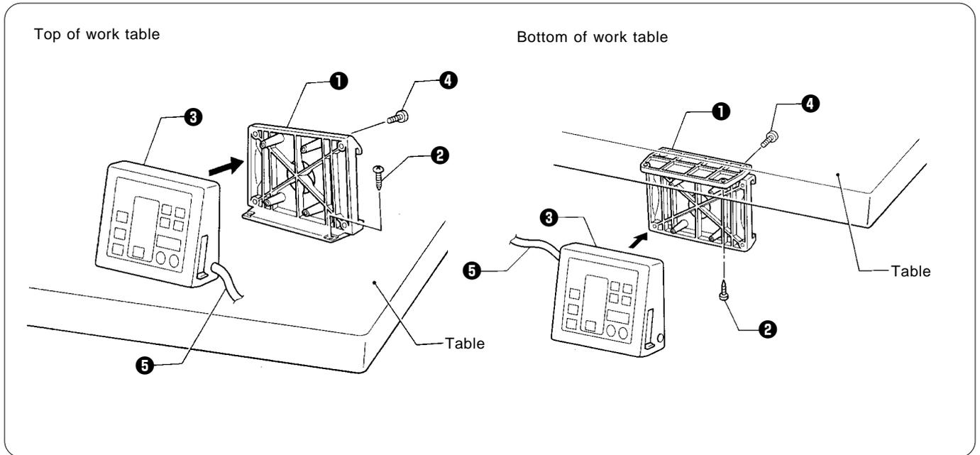
1. Install the rear frame **1** to the work table (top or bottom) with the four wood screws **2**.
