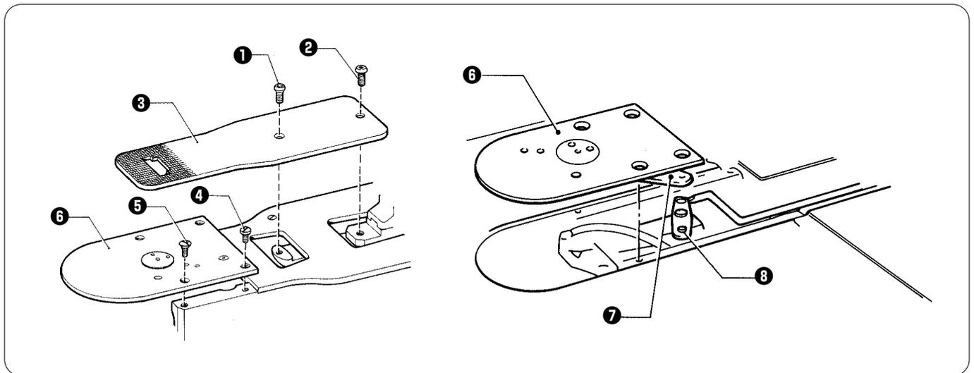
1. Open the large shuttle hook cover, remove the screws **1** and **2**, and then remove the feed plate **3**.
