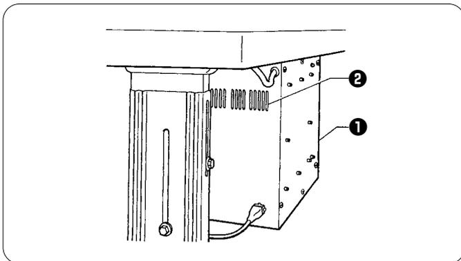
Use a vacuum cleaner to clean the filter in the air inlet port ❷ of the control box ❶ at least once a month.
