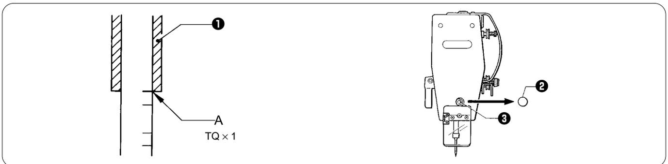
Turn the machine pulley to move the needle bar to the lowest position. Then remove the rubber plug **2**, loosen the set screw **3** and then move the needle bar up or down to adjust so that the highest reference line (reference line A) is aligned with the lower edge of the needle bar bush **1**.
