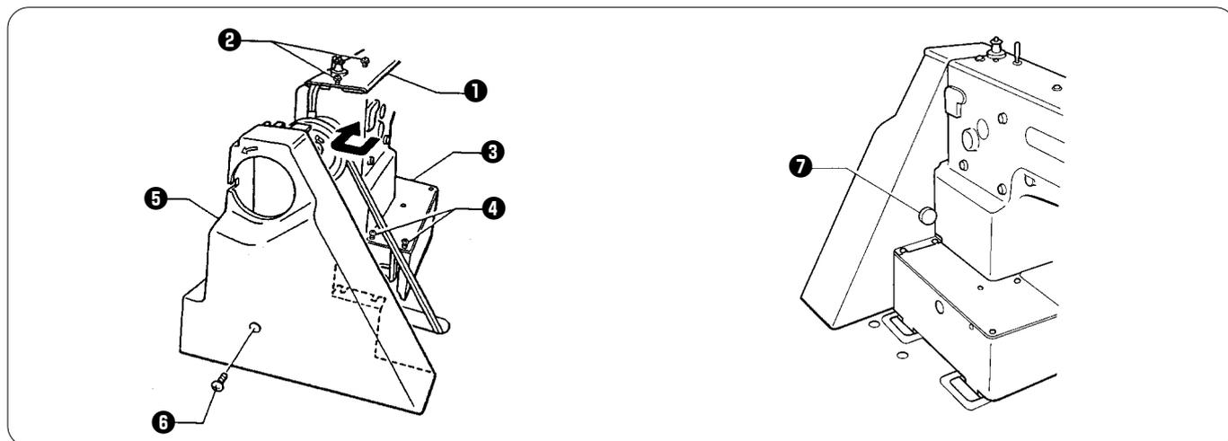
1. Loosen the two screws **2** of the upper cover **1** and the two screws **4** of bed cover L **3**.
