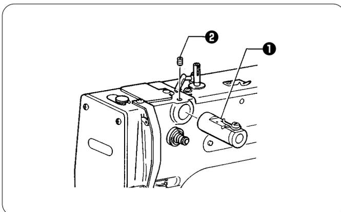
1. Remove the rubber plug, and then push the liquid cooling tank **1**.
