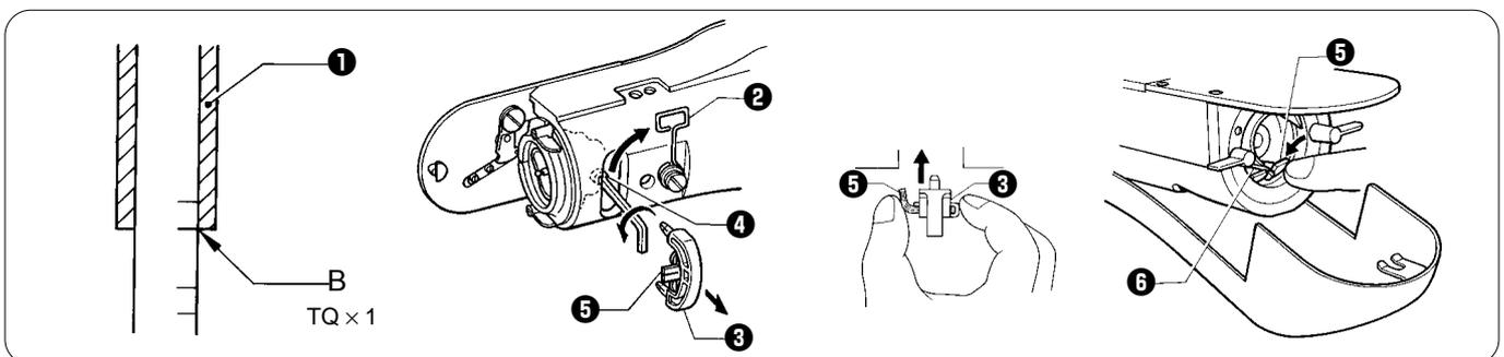
Adjust the needle bar lift amount as described below so that the tip of the rotary hook is aligned with the center of the needle when the machine pulley is turned to raise the needle bar from its lowest position until the second reference line from the top of the needle (reference line B) is aligned with the lower edge of the needle bar bush **1**.
