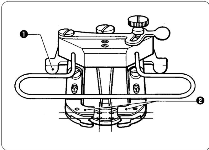
1. Press the cam plate **1** to open the button holder **2**.
