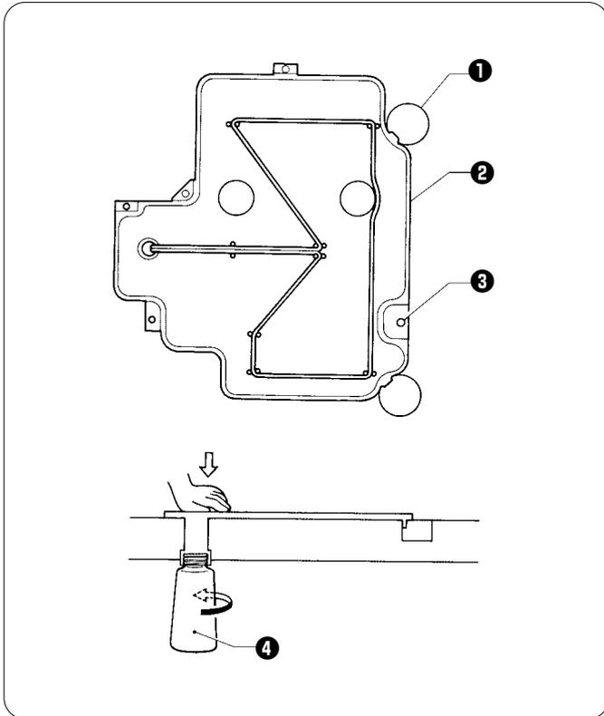
1. Insert the tabs of the oil pan **2** into the holes for the cushions **1**, and then secure it in place with the five nails **3** so that the oil pan **2** is not at an angle.
