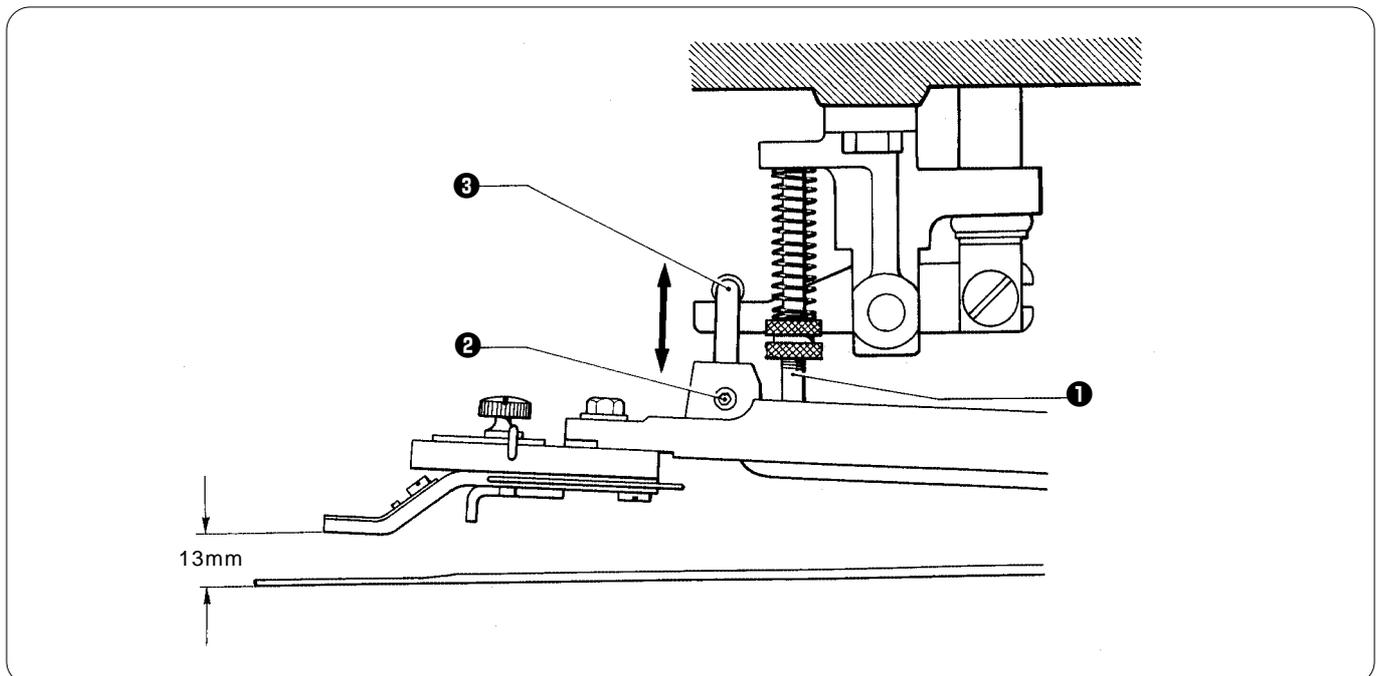
Remove the button clamp presser spring ❶, loosen the screw ❷ and adjust the button clamp holder hook ❸ by moving it up and down.
