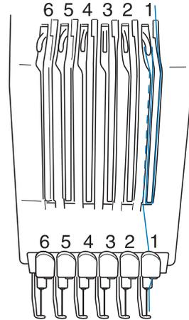
**3** Pass the thread through the hole in the number 1 upper thread guide.
