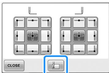
► The needle bar is positioned in the lower-left corner of the pattern. The embroidery frame moves so that the needle is positioned correctly.
