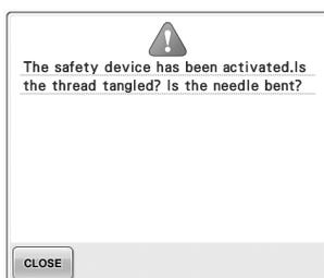
The motor has locked up due to tangled thread or for other reasons related to thread delivery. If the thread is entangled in the bobbin case, clean the race, and then oil it. (Refer to page 247 and 251.)
