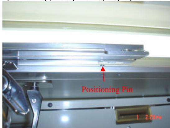
3. Open the two fixed levers and move the fixing pins to the outside to take them out from the pantograph.
