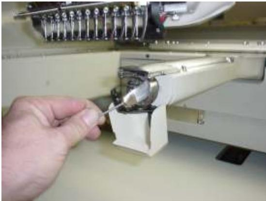
2. Insert bobbin cases in to rotary hooks. Make sure bobbin thread is not over 2 inches long. Close bobbin case covers.
