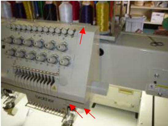
3. Remove the right end cover by removing the two lower screws and loosening two upper screws. Plus removing a screw on the cover behind the head.
