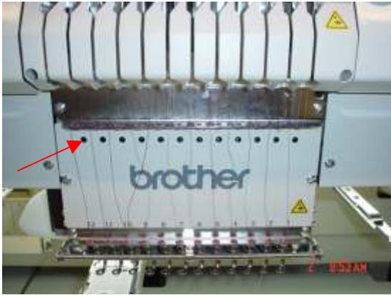
*Note: Cover in photo has been removed for illustration of where to lubricate.*
