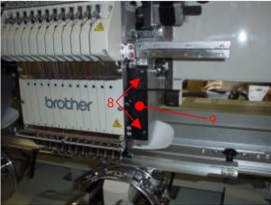
13. Grease the cam groove of the thread take-up driving cams.
