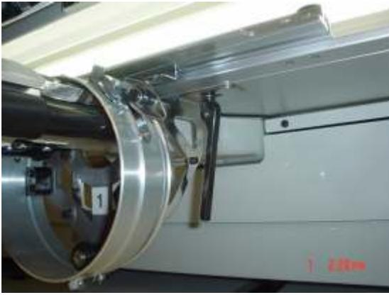
6. Install the black thumbscrews on to the pantograph. Adjust centering of cap frame assembly left to right before tightening thumbscrews.
