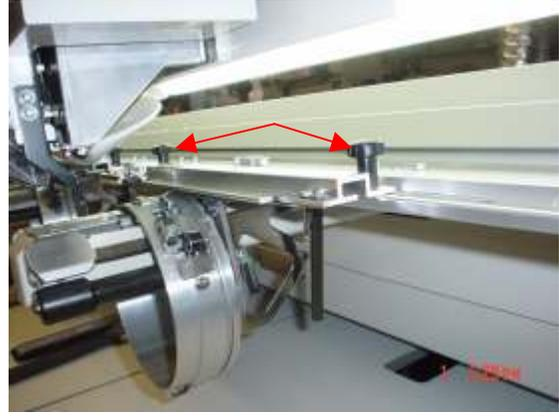
6. Flip mode switch on machine to CAP. Turn power ON.
