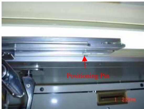
4. Hold the fixed lever as shown and insert in to the hole underneath the pantograph. Push up and toward the inside until it stops. Then lock the fixed lever by pushing down. Do this to the other side.
