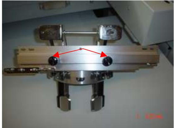
3. Lift up on the cap frame sash so that the positioning pins fit into the oval holes and lower on to the pantograph.
