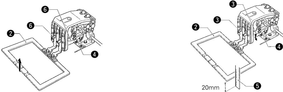
1. Turn on the air, and then press the work clamp lifter switch ① while turning it clockwise, to raise the work clamp ②.
