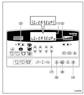
After the grease has been applied, carry out the following procedure to reset the cumulative time between grease applications.
