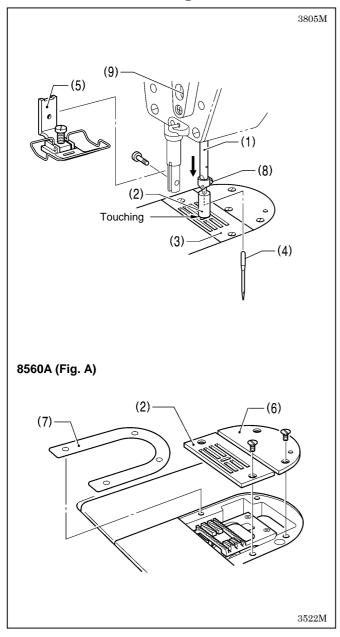
With the accessory needle bar height gauge (2) installed to the needle bar (1), adjust so that the needle bar height gauge (2) is touching the top of the needle plate (3) when the needle bar (1) is at its lowest position.
