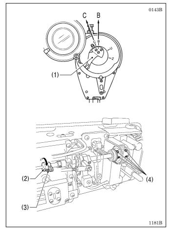
The feed amounts for reverse stitching and condense stitching are set using the condense dial (1).
