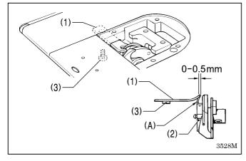
Adjust so that the end of the bobbin case holder position bracket (1) is 0 to 0.5 mm back from end (A) of the inner rotary hook (2).
