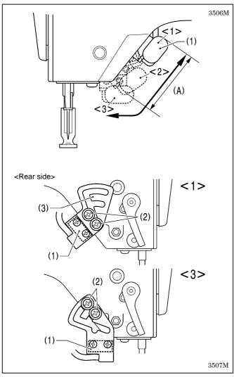
The installation position of the actuator (1) can be adjusted as shown in the illustration.
