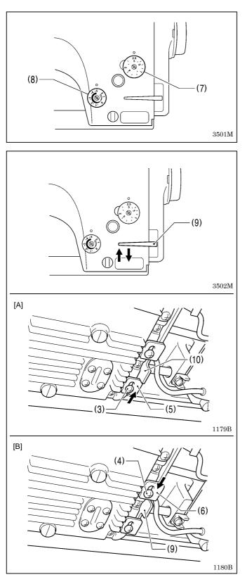
5. Turn the stitch length dial (7) and the condense dial (8) to the maximum feed amount for the feed dog being used. (Set the condense dial (8) to a negative number.)
