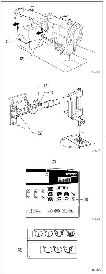
Adjust the position of the needle so that it is in about the center of the slot in the needle hole when the power is turned on and the zigzag width and zigzag base line position have both been set to 0 mm at the operation panel.
