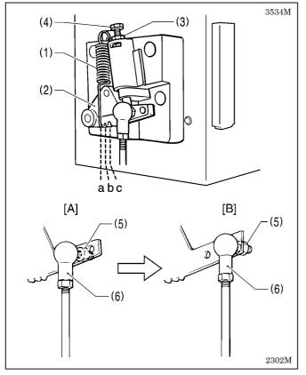
When sewing stretch materials and materials with long pile, you can make minute adjustments to the floating amount for the presser foot (1) in accordance with the material.
