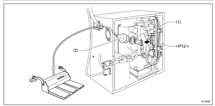
1. Insert the foot plug (1) into connector <P12> on the main P.C. board.
