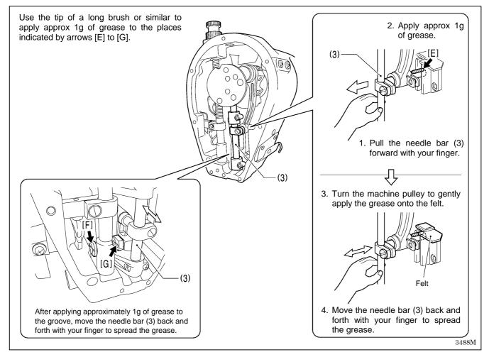
After applying grease in the places indicated by arrows [A] to [G] above, carry out the reset operation described below.
