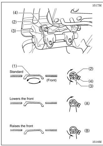
The standard angle for the feed dog (1) is for the top of the needle plate to be parallel with the top of the feed dog (1) (for the 8550A) or raised slightly at the side closest to the operator (for the 8560A) when the feed dog (1) is raised to its highest position above the needle plate. (With the  $\bigcirc$  mark on the feed bracket shaft (2) aligned with the mark on the feed rocker bracket arm (3)).
