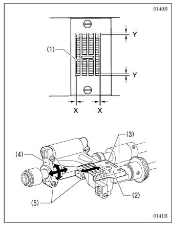
Adjust the sideways clearances X between the feed dog (1) and the needle plate so that that are approximately equal. Adjust so that the clearances Y between the front and back of the feed dog (1) and the needle plate are approximately equal when the machine pulley is turned until the feed plate (2) is moved to its furthest forward position and also when it is moved to its furthest back position.
