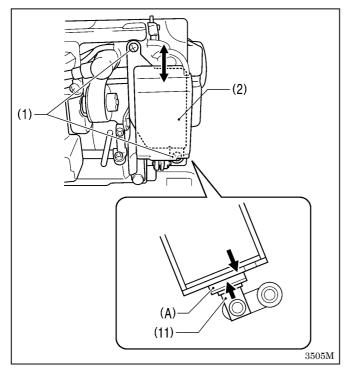
9. For sewing machine models and specifications other than 8550A-031, push the reverse stitching lever (9) down all the way (so that the plunger (11) of the quick reverse solenoid has moved to its highest position), and then tighten the two screws (1) at the position where the quick reverse solenoid (2) is touching to top of section (A) of the plunger (11).
