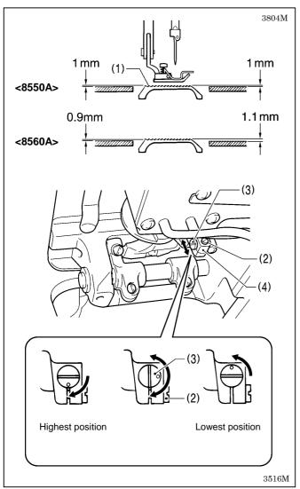
The standard height of the presser foot (1) is 6 mm when the presser foot (1) is raised by means of the lifting lever (2).
