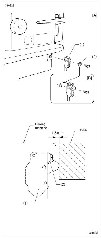
The safety switch (1) is normally installed as shown in figure [A].
