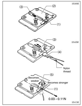
Adjust the tension of the plate spring (1) so that the tension is 0.03 to 0.11 N when the plate spring (1) is pulling the lower thread (nylon thread: 100D 1 X 3 (Z)) after thread trimming.
