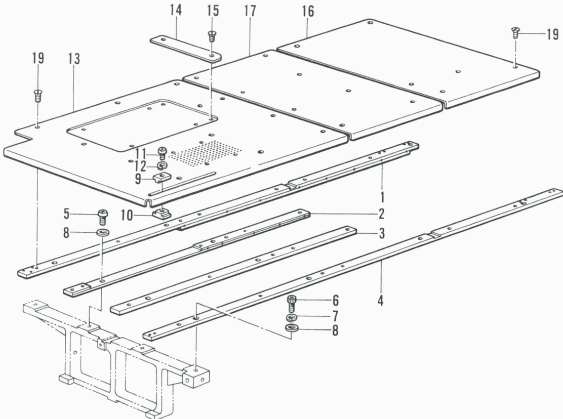
F. 糸切れ感知関係 /Thread breakage detector mechanism /Fadenbruchfühler /
