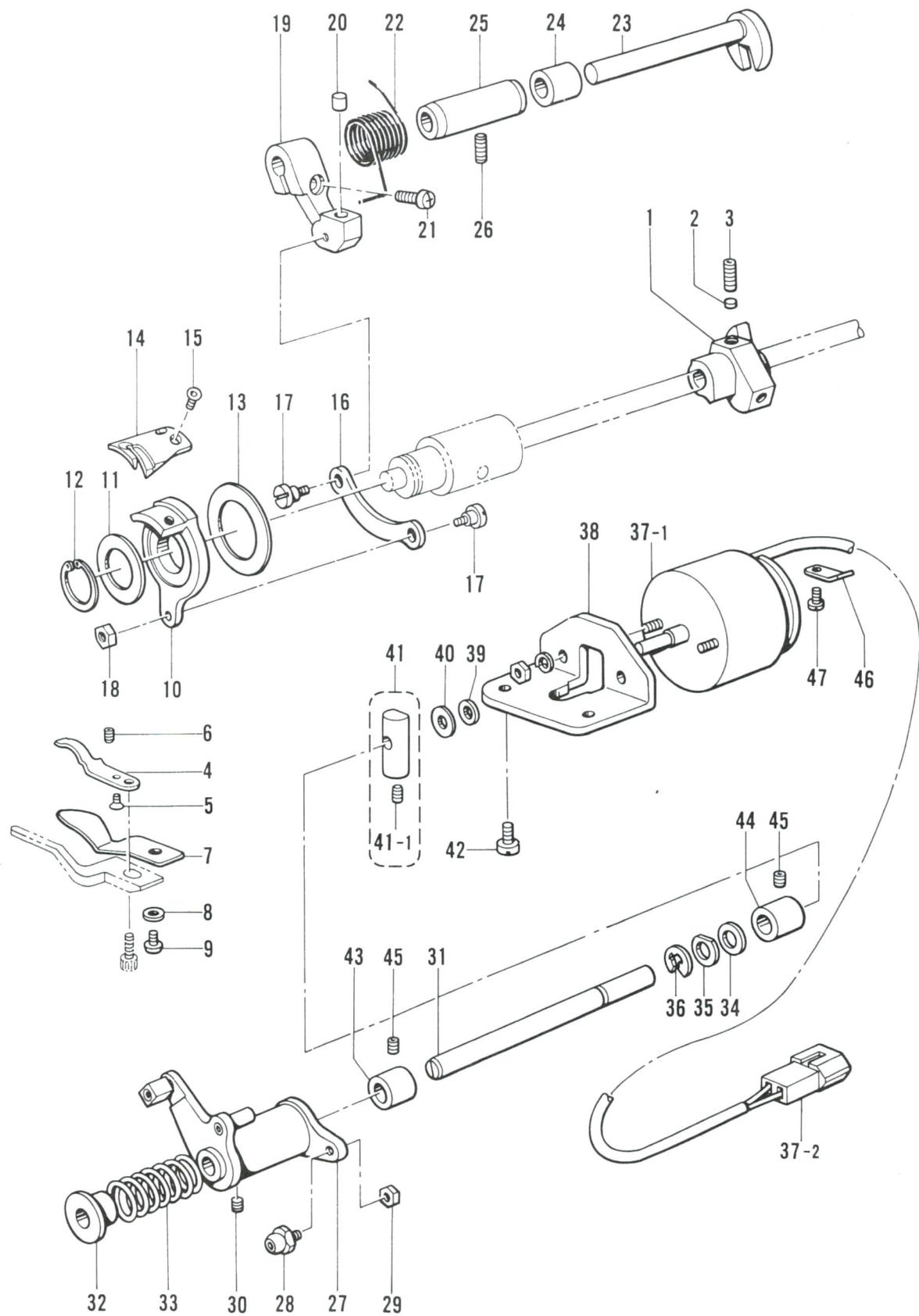
Q. 糸巻関係 / Bobbin winder mechanism / Spuler /
