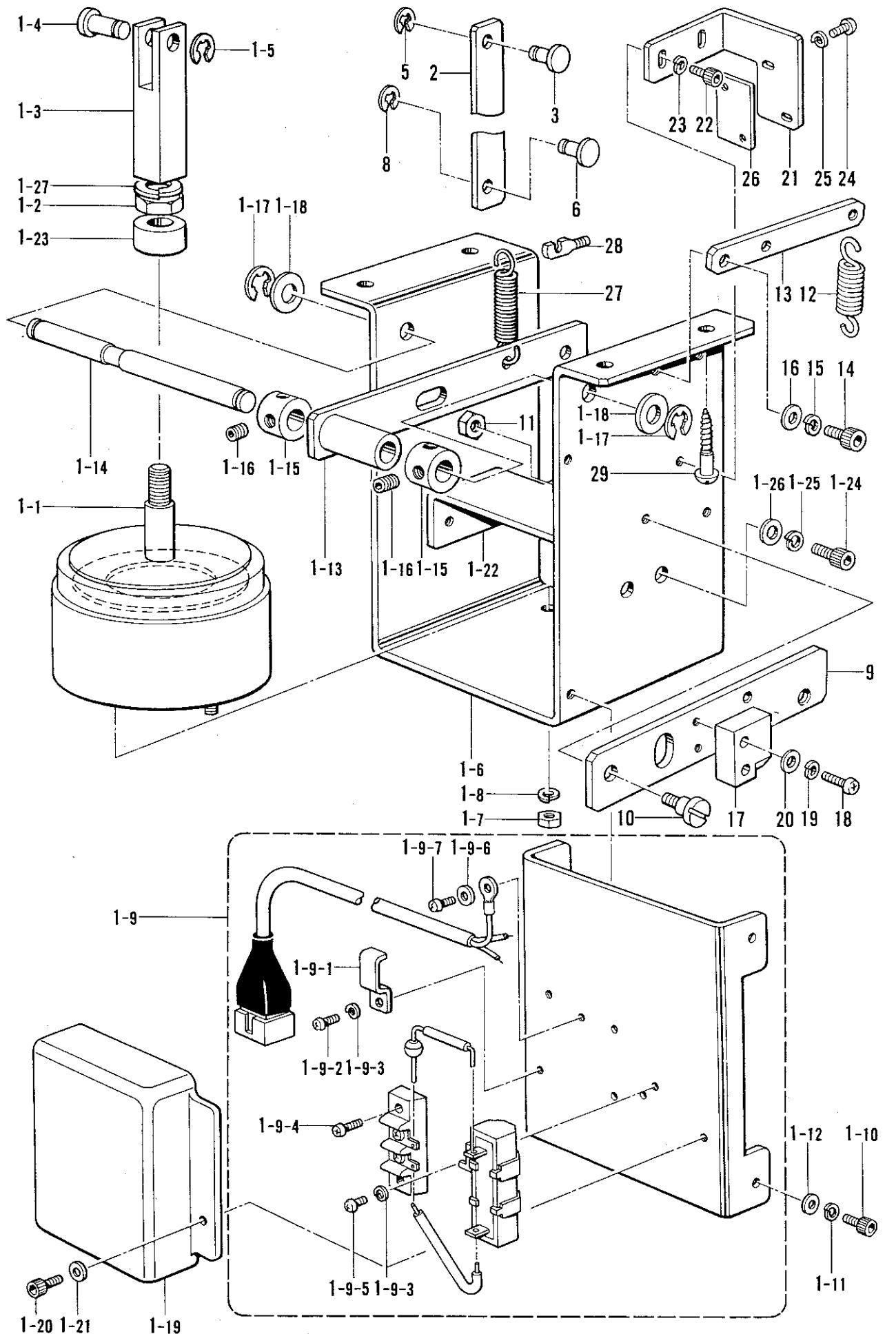
N. 起動装置関係/Starting device mechanism/Startvorrichtung/
