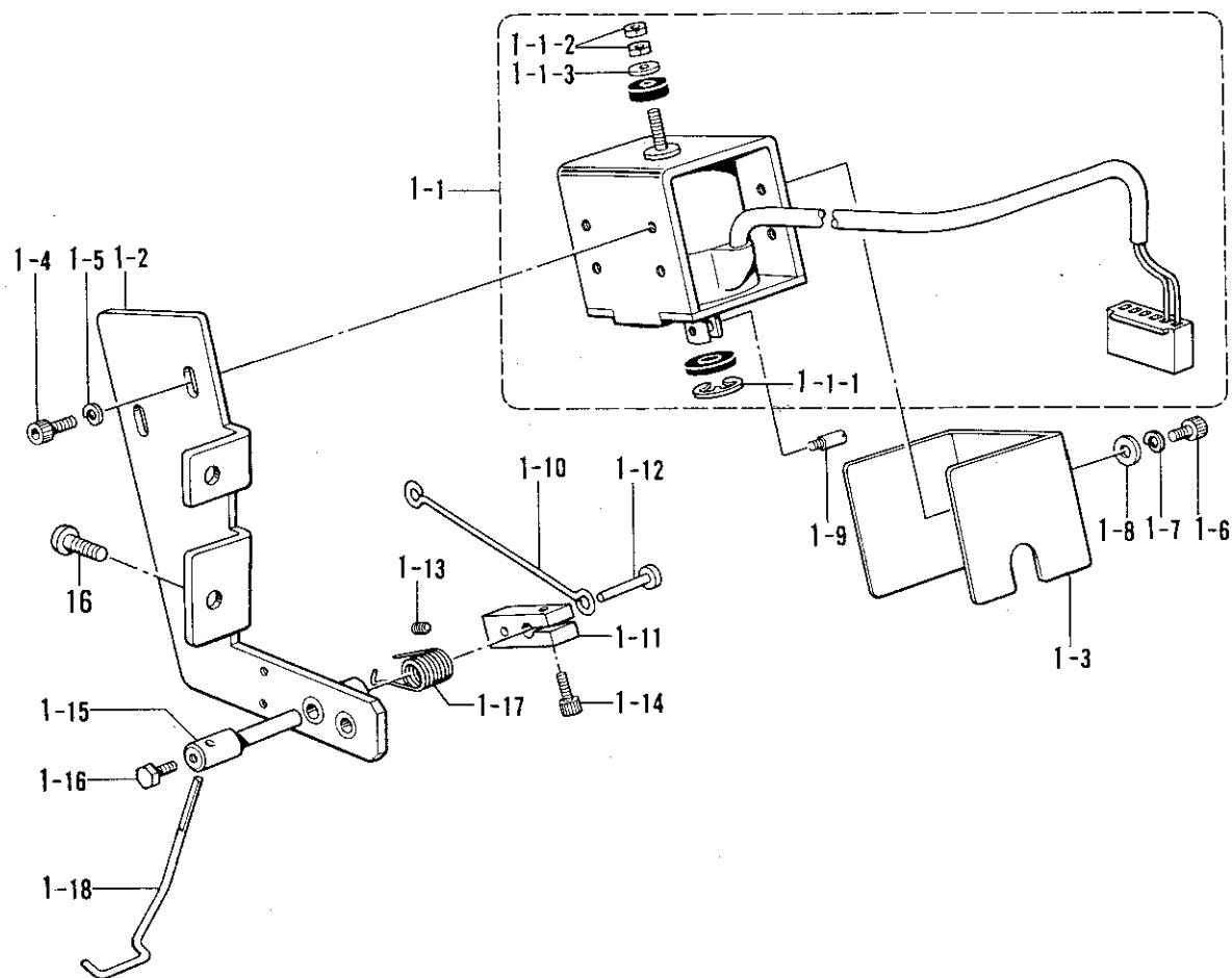
K. 糸サバキ関係/Loop spreading mechanism/Schleifenzieher/Etirement de boucle/Ensanche de bucle
