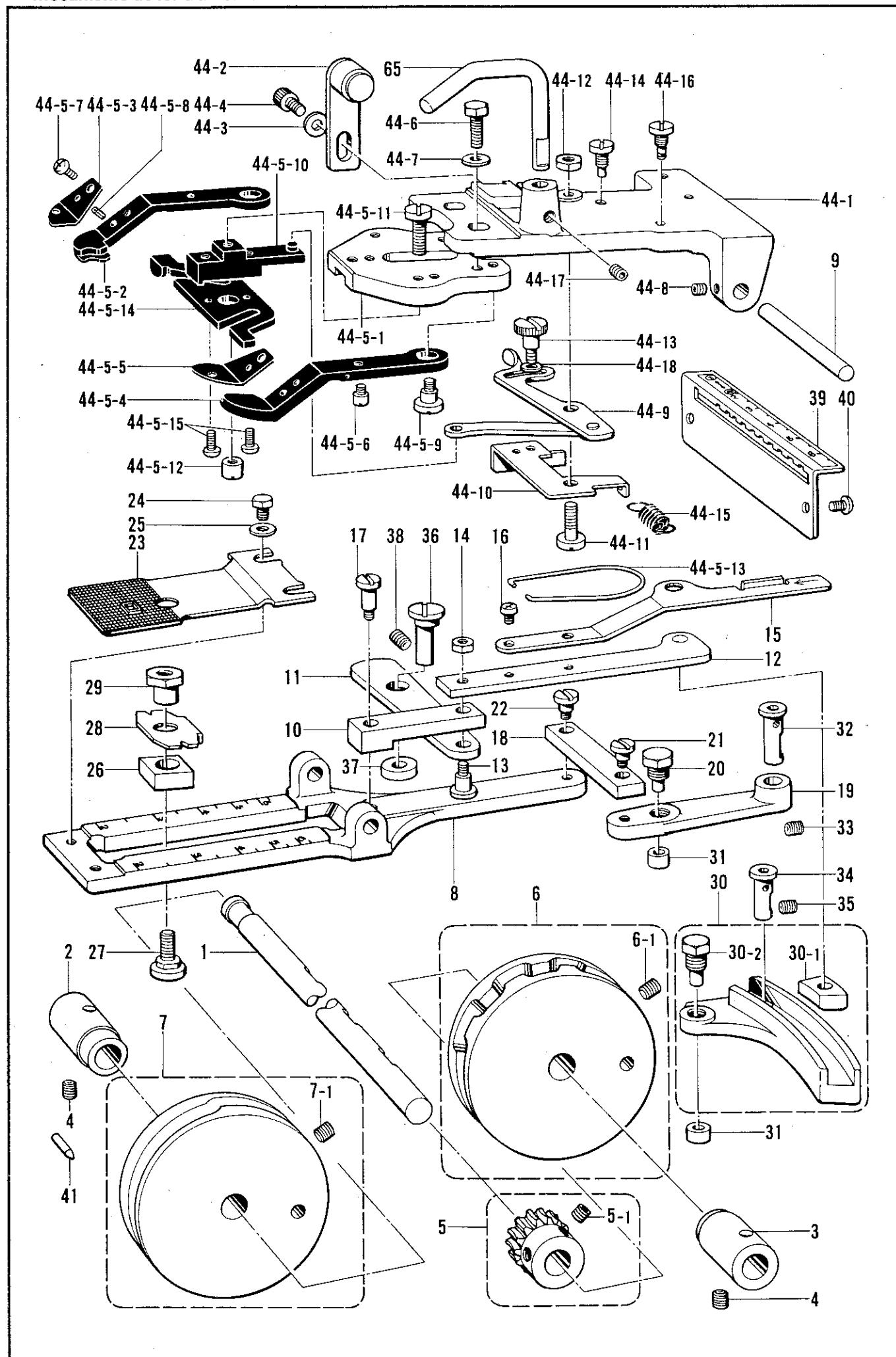
E. 送り関係/Feed mechanism/Transportvorrichtung/
