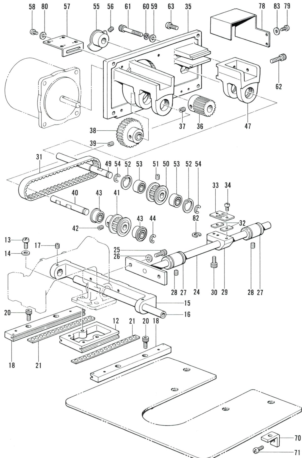
**C2. 送り関係 / Feed mechanism / Transportvorrichtung /
