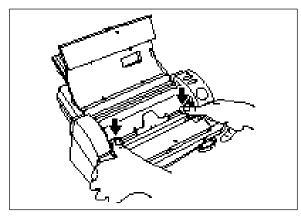
(4) Install the new film cartridge carefully.
