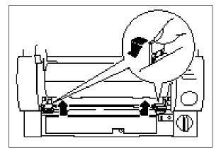
(4) Push the yellow colored tab of side cutter unit to release the lock as illustrated.
