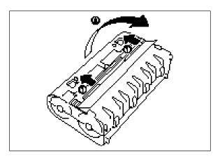
(2) Open the shutter of the film cartridge by sliding the shutter in the direction of the arrows until it locks into place. Open the film cartridge by gently separating the clear top cover from the gray bottom cover as indicated by the arrow on the clear top cover.
