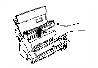
(3) Remove the film cartridge carefully.
