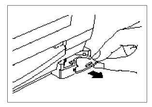
Corner Cutter Tray (Corner cutter tray CC-1) (1) Remove the corner cutter tray as illustrated.
