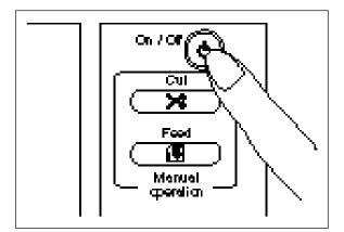
(3) Press the power switch on the control panel to turn it on. The green **Start** button will light up. If the machine does not respond, check the connection of the AC adapter.
