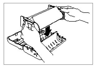
(4) Take the new roll of film from the sealed package. Holding the yellow colored plastic side holders of the film roll. Set the film into the cartridge as illustrated. The film can only be placed into the cartridge in the proper direction.
