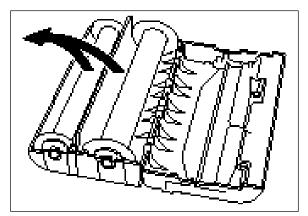
(3) Remove the old film roll from the cartridge.
