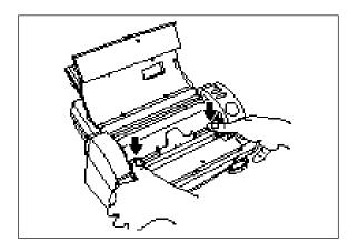
(4) Return the roller holder to the original position and press the roller holder lock buttons (purple color) as illustrated. You will hear the roller holder click into place. Press the roller holder further to secure the roller unit.
