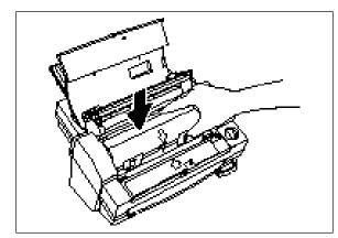
(4) Remove the film cartridge from the machine.
