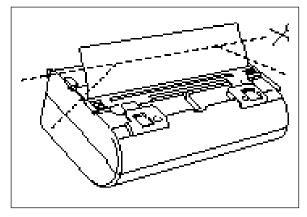
(8) Check the position of the top edge of film. It should be aligned with the cutting line of the cartridge. If any film extends beyond the cutting line, cut away the access film as illustrated before installing the cartridge.
