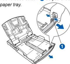
f. Gently adjust the paper side guides to the paper with both hands. Make sure the paper side guides touch the edges of the paper.
