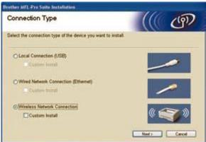
Note If you want to install the PS driver (Brother's BR-Script Driver), choose Custom Install and then follow the on-screen instructions. When the Select Features screen appears, check PS Printer Driver, and then continue following the on-screen instructions.
