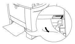
• If a paper jam occurs when using A6 size paper, remove the jammed paper, turn over the stack of the paper in the paper cassette, and print it again.
