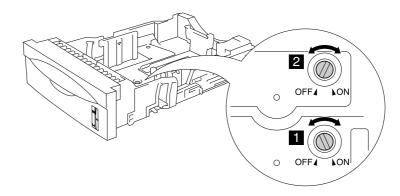
The switches shown in this illustration are in the default setting position.
