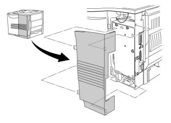
☞ 3. Unscrew the three screws in the order shown, and then remove the metal plate.
