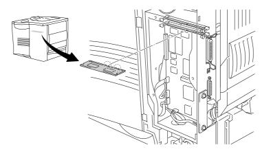
☞ 6. Press the DIMM straight into the slot (press firmly). Make sure the locks on each side of the DIMM snap inward into place. (To remove a DIMM, the locks must be released.)
