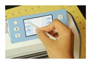
Select the icon on the top left of the screen. This is where we can erase parts of the image we scanned in because it includes some info we don't want the machine to cut out.
