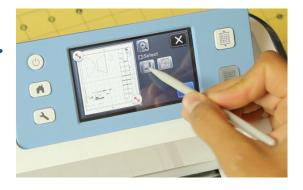
Select the first icon under the word "Select." You will see a box form around your scanned image and on each diagonal corner, there is a circle with red arrows inside. These are handles that you can move around to frame out the items you'd like to bulk delete.
