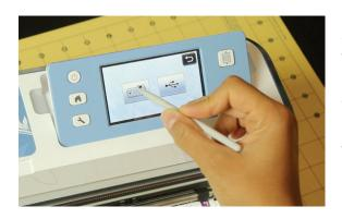
Select the machine icon to save the new design to the machine's internal memory. (You also have the option of saving it to an attached USB device.) Follow the prompts and click "OK."
