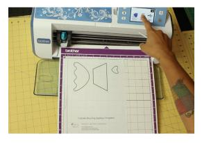
Select the "Scan to Cut Data" icon, load your mat and hit "Start/Stop." The machine will scan the mat and display your appliqué design on the screen.
