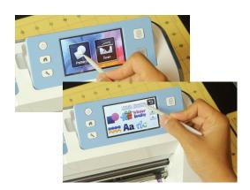
From the main screen, select "Pattern," then "Saved Data," and locate and select the file you just saved in the machine's internal memory.
