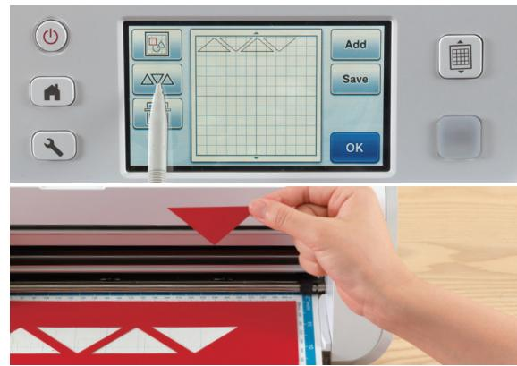
**Tip** The Auto Layout function can help save paper by automatically calculating the most efficient layout to use when you cut multiple pieces.
