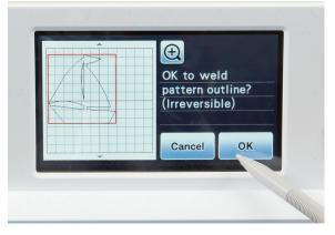
When making pieces using built-in patterns like the boat and airplane that are composed of separate parts, the Unify editing function is handy for joining them together.
