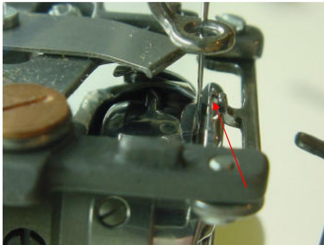
7. Position tip of rotary hook stopper so that a gap of approximately 1 – 1.5mm is maintained from rotary hook bobbin basket as indicated by the red arrow and tighten screws.
