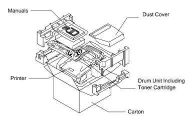
Fig. 5-28 Repacking the Printer
