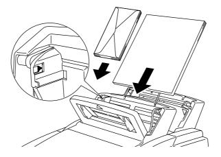
Fig. 2-5 Loading Paper or Envelopes in the Feeder
