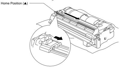
Fig. 5-23 Cleaning the Primary Corona Wire
