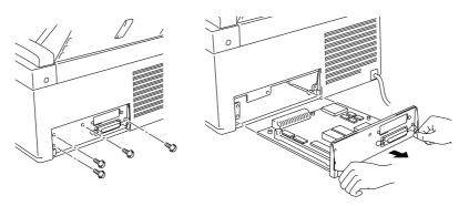
Fig. 4-4 Remove the main controller board
