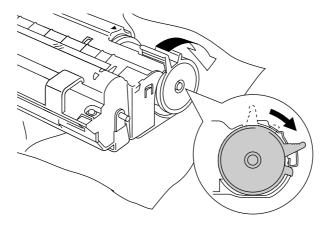
Fig. 5-8 Turning the Lever to Open the Shutter
