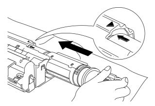
Fig. 5-7 Installing the Toner Cartridge into the Drum Unit
