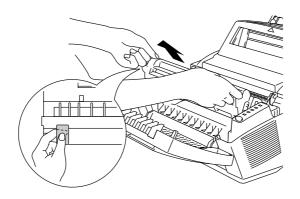
Fig. 5-26 Removing the Drum Unit Assembly
