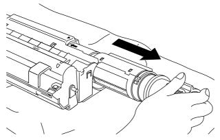
Fig. 5-5 Removing the Old Toner Cartridge
