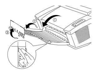
Fig. 2-10 Opening the Output Tray and **Extending the Extension Support Wire**
