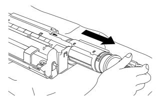
Fig. 5-12 Removing the Toner Cartridge
