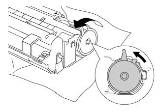
Fig. 5-4 Turning the Lever to Close the Shutter
