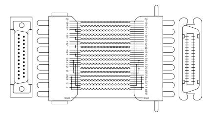
Fig. A-1 Parallel Interface Cable
