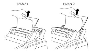
Fig. 6-3 Paper Jam in the Feeders
