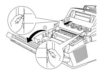
Fig. 5-24 Cleaning the Feeder 1 Paper Feed Rollers
