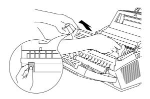
Fig. 5-2 Removing the Drum Unit
