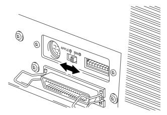
Fig. 4-1 Selecting the RS-422A (Apple) or RS-232C (IBM) Serial Interface
