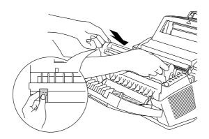
Fig. 5-15 Installing the Drum Unit
