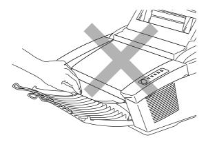
Fig. 6-7 Do Not Pull the Jammed Paper from the Output Tray
