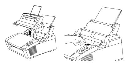
Fig. 6-4 Paper Jam under Feeder 1
