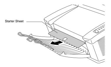
Fig. 5-16 Ejecting the Starter Sheet
