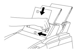
Fig. 2-9 Moving the Paper Guide
