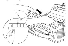
Fig. 5-10 Removing the Drum Unit
