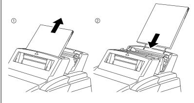
Fig. 2-7 Loading Paper in Feeder 2
