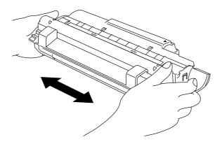
Fig. 5-13 Shaking the Drum Unit
