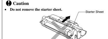
Fig. 5-14 Do Not Remove the Starter Sheet
