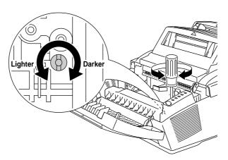
Fig. 5-17 Adjusting the Print Density Dial
