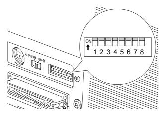
Fig. 4-2 Setting the Serial Interface Parameters
