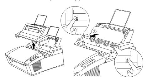
Fig. 5-25 Cleaning the Feeder 2 Paper Feed Rollers
