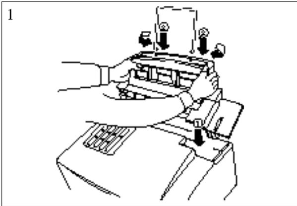
Replace the sheet feeder onto the printer.
