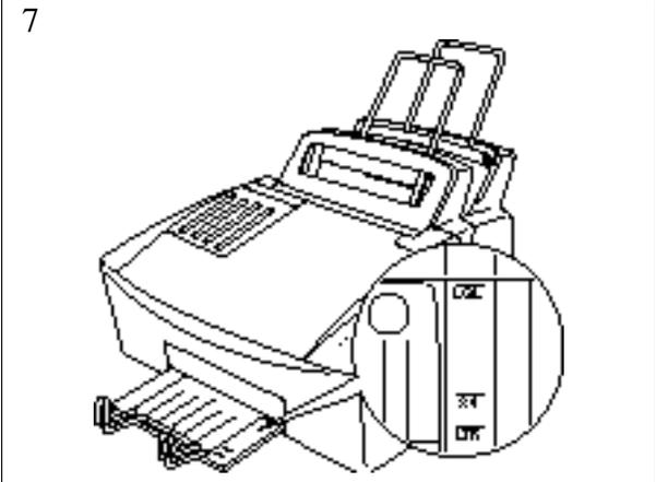
Pull out the Output Tray and adjust the tray position for the loaded paper as follows:
