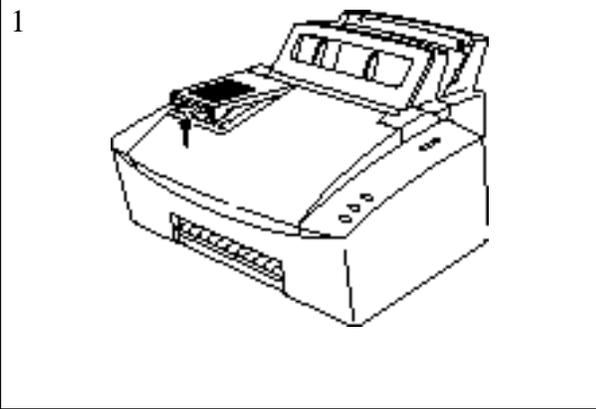
Remove the tapes, and 2 pieces of Styrofoam supporting the print head then open the ink reservoir cover.
