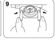
Push the latch levers into their locked position. Replace the bobbin case.
