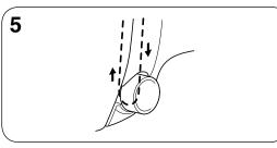
Pass the thread into the thread tension discs or behind the thread tension dial from the right to the left.
