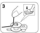
While holding the end of the thread, press the foot controller to begin winding the thread. Cut the thread from the top and proceed winding.
