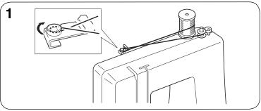
Pull up on the thread spool pin to lengthen the height. Place the thread spool on the pin and pass the thread around the bobbin winder pre-tension disc.
