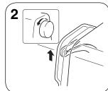
Raise the thread take-up lever to its highest position by turning the
