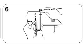
Grasp the thread on both sides of the tension disc and pull to
