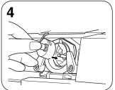
Holding the bobbin case by the latch, align your finger with the top opening of the shuttle race, insert the case into the shuttle race and release the
