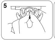
pull the latch and remove the bobbin
