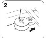
Pass the thread through the hole on the bobbin from inside. Use upper hole, not both. Place on bobbin shaft and slide to the right.
