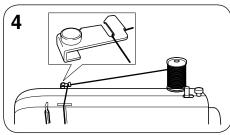
Pass the thread through the thread guide and down the right channel on the front of the machine.
