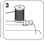
Place the thread spool on the spool pin. (Don't forget to pull up the pin)
