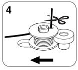
When the bobbin starts to spin slowly and becomes full, release the foot controller. Cut the thread, slide the bobbin winding shaft to the left and remove the bobbin.
