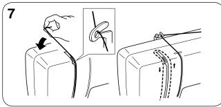
Guide the thread up the left channel, clear to the back of the opening around Thread the needle from front to back and pull the take-up lever and back down the left side of the channel to thread the
