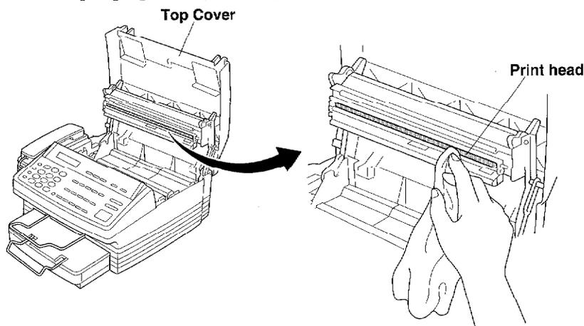
**Helpful Hints** If the scanner and the print head are dirty, the quality of the transmission or reception image, and copy becomes degraded. Use the above procedure to clean these parts frequently.
