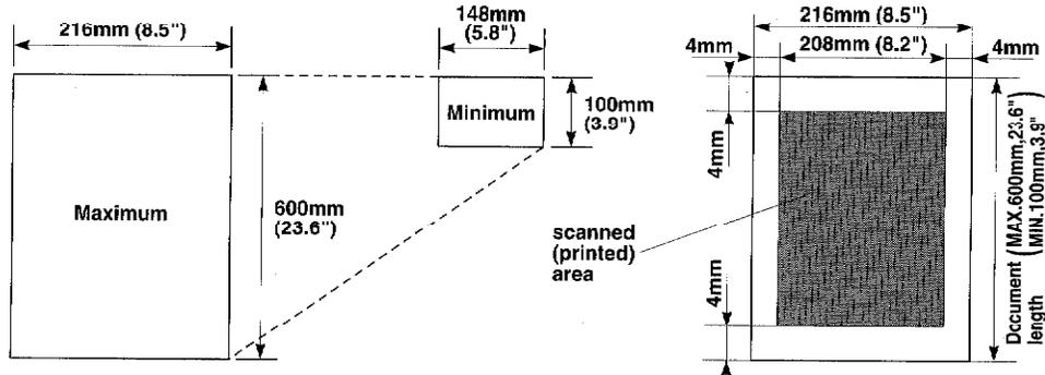
The size of the documents you want to send by fax should not be larger (or smaller) than your fax machine can accommodate. The documents should each be between 148 and 216 mm (5.8 and 8.5 inches) wide and between 100 and 600 mm (3.9 and 23.6 inches) long.
