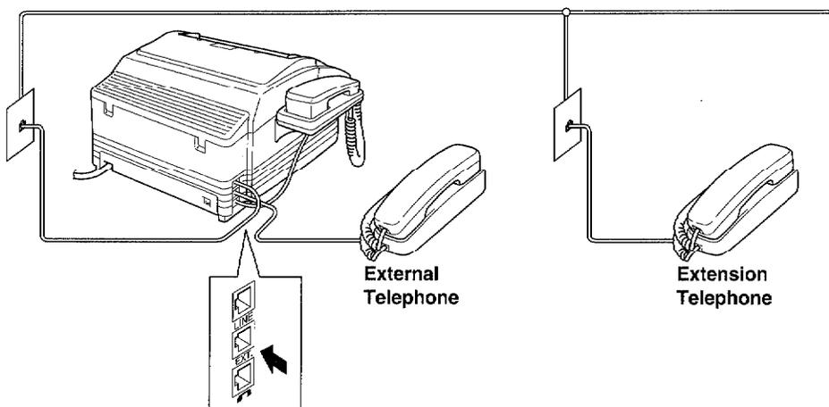
If the external telephone is in use, the warning message "EXT. TEL IN USE" will be displayed on the fax LCD. When the handset on the fax machine is picked up, an alarm will sound. You can disconnect the external phone and switch to the fax machine's handset by pressing **HOOK**.
