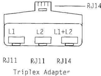
**Installing a Fax Machine, Two Line TAD and Two Line Telephone**
