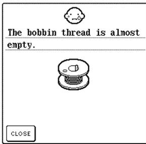
This message is displayed when the bobbin thread is running out.
