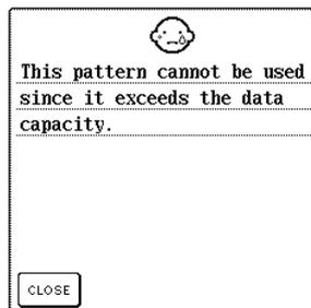
This message is displayed when you try to retrieve a pattern saved with the number of stitches or the number of colors exceeding the specified limits.
