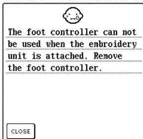
This message is displayed when the foot controller is pressed while the embroidery unit is attached.
