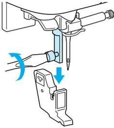
**3** Set the operation lever of the walking foot so that the needle clamp screw is set between the fork, and position the walking foot on the presser foot bar.
