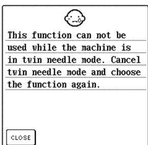
This message is displayed when the machine is set for twin needle sewing and a pattern that cannot be sewn with the twin needle is selected.
