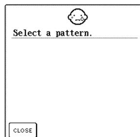
This message is displayed when the "Start/Stop" button, "Reverse/Reinforcement Stitch" button or
