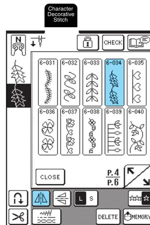
→ The second pattern is flipped on a vertical axis.
