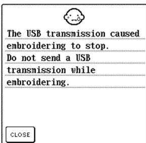
If data is being written to or deleted from "Removable Disk" on the connected computer during sewing, the machine stops and this message is displayed. When the USB transmission is completed, press the "Start/Stop" button to continue sewing.
