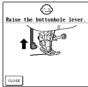
This message is displayed when a stitch other than a buttonhole stitch is selected and the "Start/Stop" button or the "Reverse/Reinforcement Stitch" button is pressed while the buttonhole lever is lowered.
