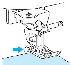
\* The presser foot remains level, enabling the fabric to be fed. Once the trouble spot has been sewn, the presser foot will return to its normal operation.
