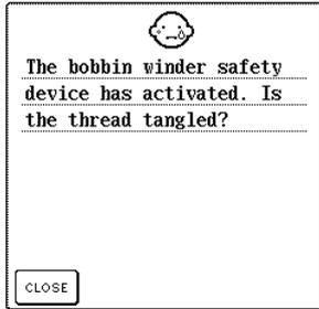
This message is displayed when the bobbin is being wound, and the motor locks because the thread is tangled, etc.
