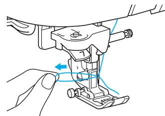
**15 Pull out about 100 mm (approx. 3-4 inches) of the thread, and then pass it under the presser foot toward the rear of the machine.**
