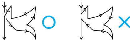
If the design is to be repeated and linked, the start point and end point of the design should be at the same height.
