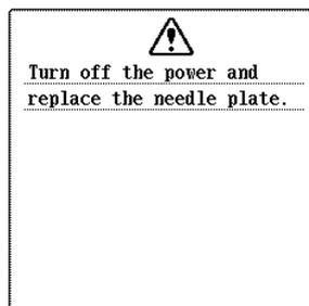
This message is displayed when you try to sew with a stitch other than a middle needle position stitch while the single-hole needle plate is installed.
