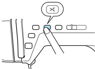
→ The needle automatically stops in the raised position.
