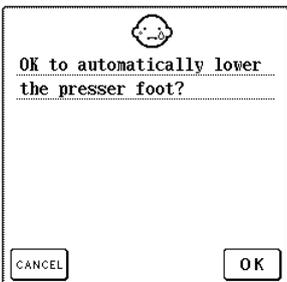
This message is displayed when
