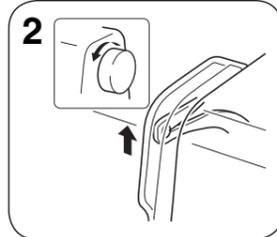
2 Raise the thread take-up lever to its highest position by turning the handwheel.
