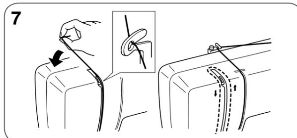
7 Guide the thread up the left channel, clear to the back of the opening around the take-up lever and back down the left side of the channel to thread the take-up lever.
