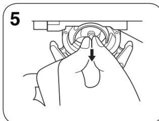
5 Remove the hook by grasping the center post and pulling out. Note its position related to the driver.
