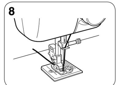
8 Thread the needle from front to back and pull out about 5 cm (2 inches) of thread.
