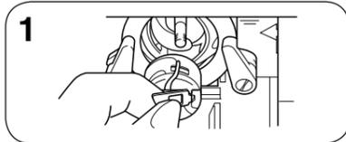
1 Raise the needle to its highest position and remove the bobbin case by pulling the latch.
