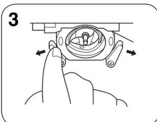
3 Slide the latch levers out from the retaining ring.
