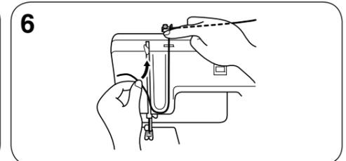
6 Grasp the thread on both sides of the tension disc and pull to ensure it is in place.
