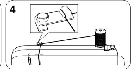
4 Pass the thread through the thread guide and down the right channel on the front of the machine.
