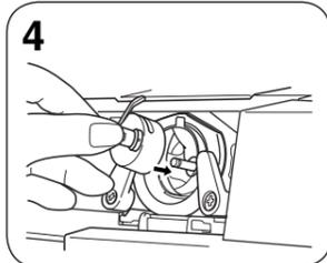
4 Holding the bobbin case by the latch, align your finger with the top opening of the shuttle race, insert the case into the shuttle race and release the latch.
