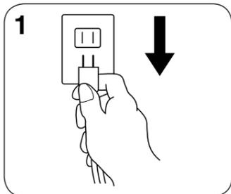
1 Remove the power plug from the outlet.
