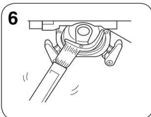
6 Remove any accumulated lint and thread with a brush.
