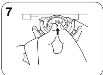
7 Grasp the center post of the hook, match the hook position opposite the driver and insert.
