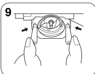
9 Push the latch levers into their locked position. Replace the bobbin case.
