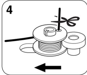
4 When the bobbin starts to spin slowly and becomes full, release the foot controller. Cut the thread, slide the bobbin winding shaft to the left and remove the bobbin.
