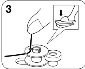
3 While holding the end of the thread, press the foot controller to begin winding the thread. Cut the thread from the top and proceed winding.
