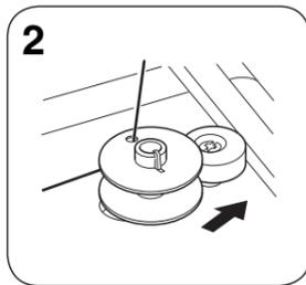
2 Pass the thread through the hole on the bobbin from inside. Use upper hole, not both. Place on bobbin shaft and slide to the right.
