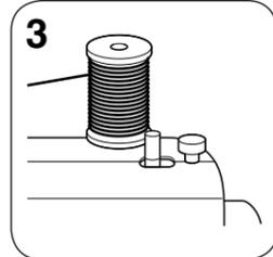
3 Place the thread spool on the spool pin. (Don't forget to pull up the pin)
