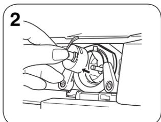
2 Raise the needle to its highest position, pull the latch and remove the bobbin case.
