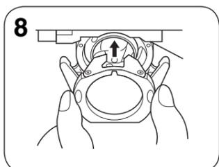
8 Insert the retaining ring with the notch up.
