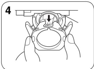
4 Remove the retaining ring.
