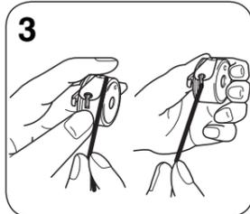
3 Pull the trailing thread through the slot, down and to the left, until it enters the delivery eye under the tension spring. **CAUTION:** Make sure you set the bobbin so the thread unrolls in the right direction. If the thread unrolls in the wrong direction, it may cause the thread tension to be incorrect or break the needle.
