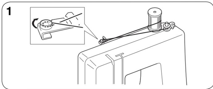
1 Pull up on the thread spool pin to lengthen the height. Place the thread spool on the pin and pass the thread around the bobbin winder pre-tension disc.
