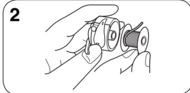
2 Hold the bobbin case as shown. Insert the bobbin with the thread coming from the bottom toward the top and the thread tail hanging out of the bobbin case.
