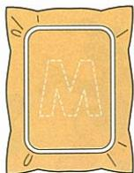
Press the START/STOP switch. The machine will sew around the position of the applique and will then stop.
