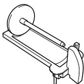
When using the extra spool pin, attach either the large or small white spool cap, depending on the size of the spool. Use the spool cap with a diameter that is slightly larger than the diameter of the spool.
