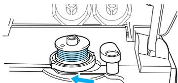
**16** Remove the bobbin from the shaft.
