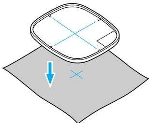
**4** Place the inner frame with the fabric on the outer frame and stretch the fabric.
