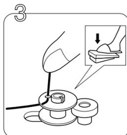
While holding the end of the thread, depress the foot controller.
