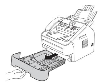
While pressing the green paper-guide release lever ①, slide the paper guides to fit the paper size you are loading in the tray. Make sure that the guides are firmly in the slots.
