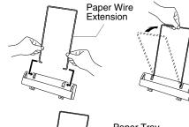
3. Attach the paper tray. Make sure the wide pins on the paper tray are inserted firmly into the pockets on the top edge of your machine.
