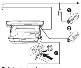
1. Extension telephone 2. External telephone 3. Protective cap
