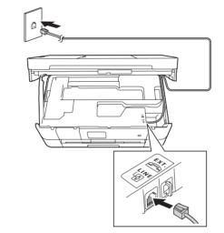
Connect the telephone line cord. Use the jack marked **LINE** and guide the cord out the back of the machine.
