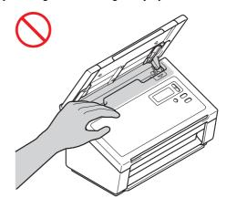
DO NOT carry the machine by holding the top cover. Doing this may cause the machine to slip out of your hands. Only carry the machine by placing your hands under the entire machine.
