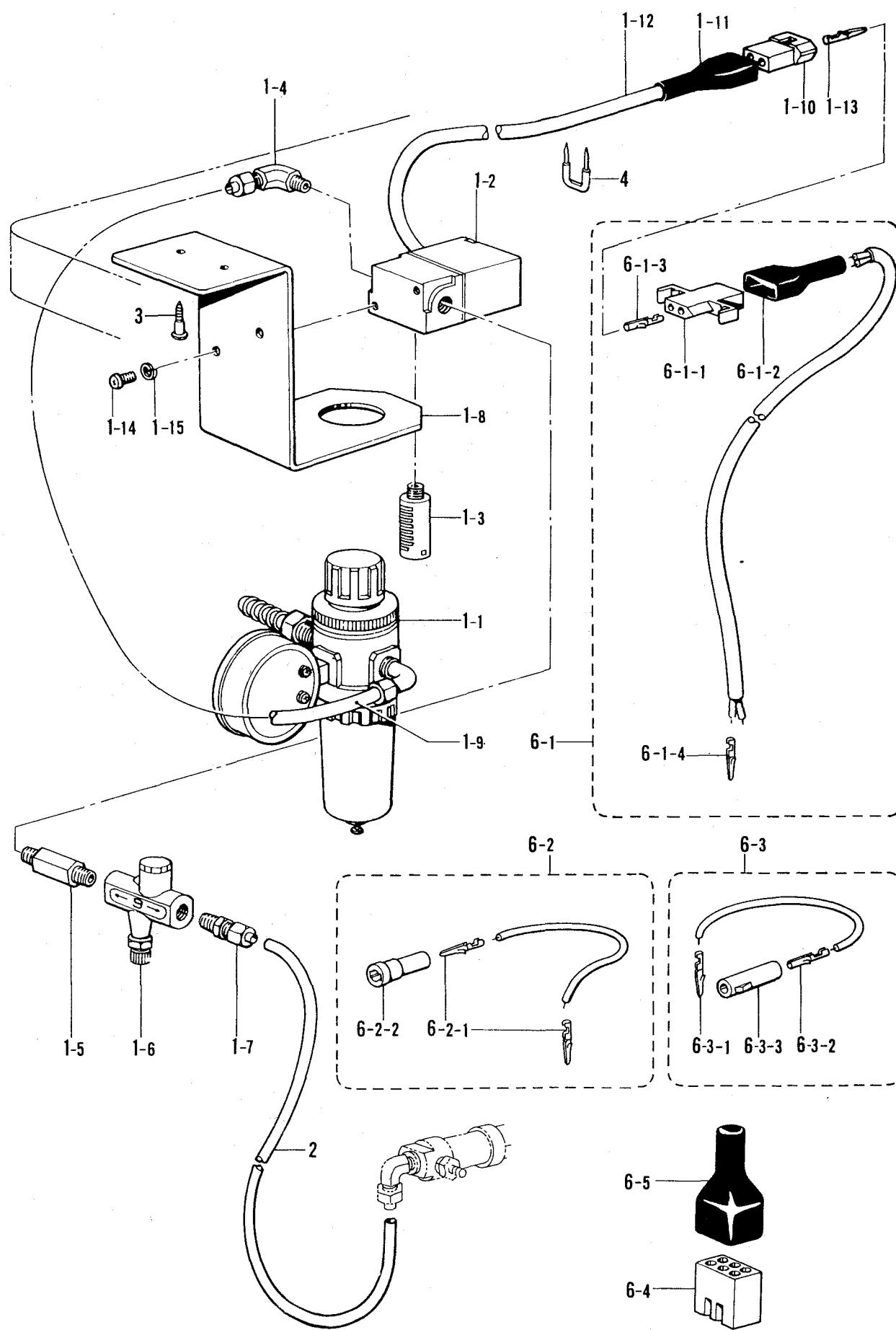
T. 空圧関係/Air pressure mechanism/Luftdruck/
