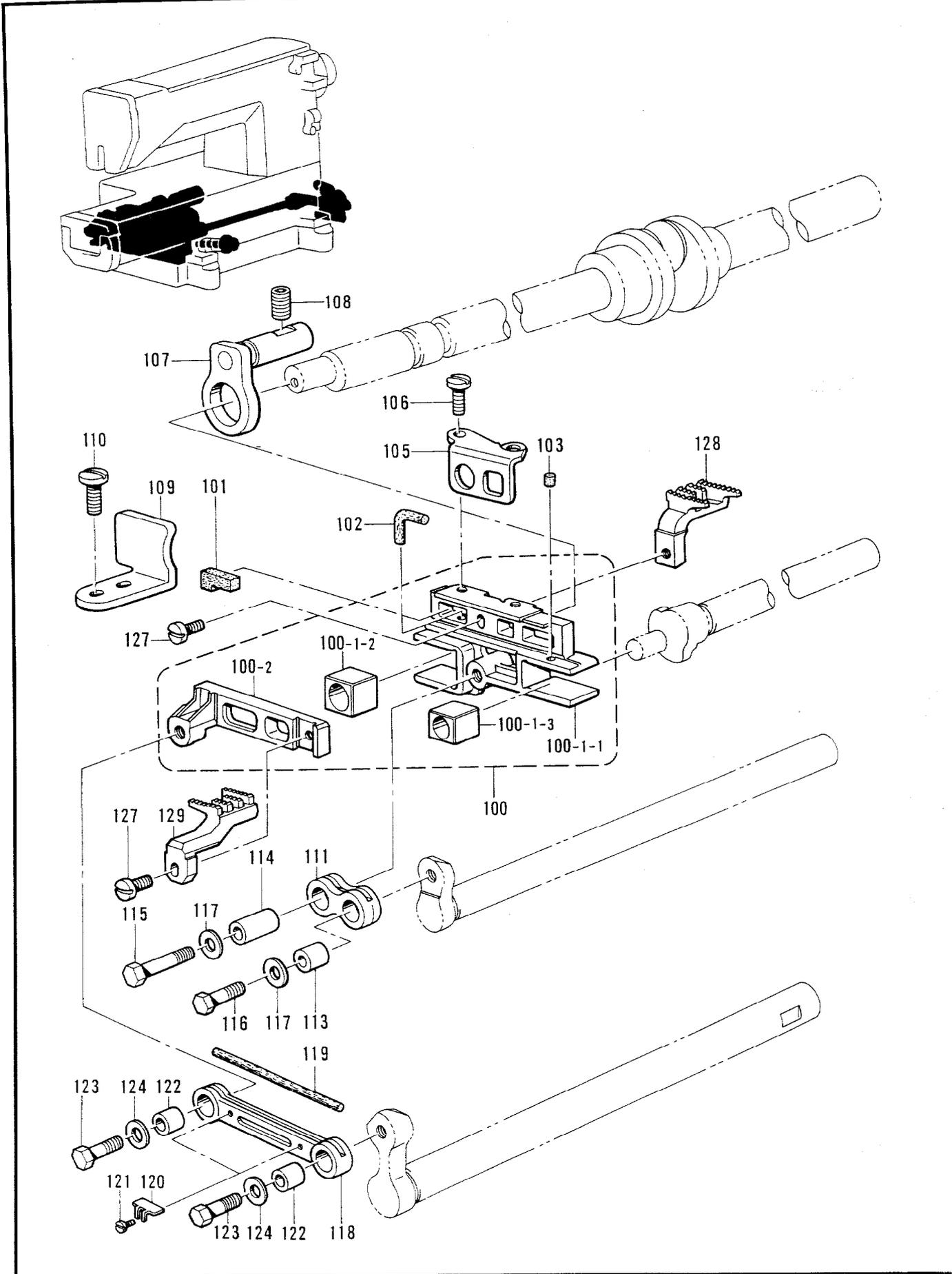
E2. 送り関係 / Feed mechanism / Transportvorrichtung /
