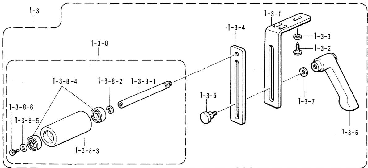
W1. 布張ローラ装置関係 / Fabric tension roller device set / Stoffspannrollervorrichtung /
