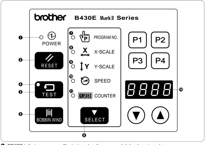
• POWER indicator ...... Illuminates when the power switch has been turned on.
