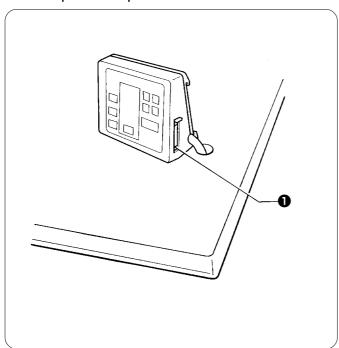
The operation panel DIP switches **1** are used to change functions which might need to be changed depending on the sewing conditions.
