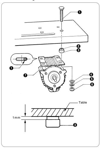
Install the motor **7** to the work table with the four accessory bolts **1**, cushions **2**, cushion collars **3**, flat washers **4**, spring washers **5** and nuts **6**. At that time, fix by setting bolts **1** a little to the right of oval hole on motor.
