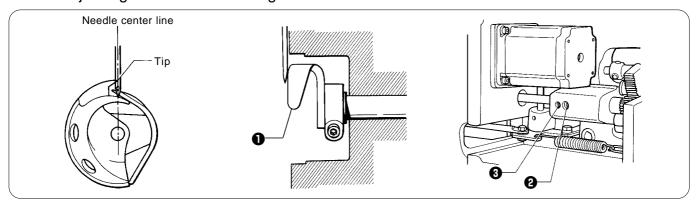
Turn the machine pulley to align the tip of the rotary hook with the needle center line. Then loosen the set screw 2 and turn the eccentric shaft 3 to adjust so that the driver needle guard 1 contacts the needle. If the needle contact pressure is too great, skipped stitches may occur. On the other hand, if the driver needle guard 1 is not touching the needle, the tip of the inner rotary hook will obstruct the needle, resulting in an excessively high amount of friction.
