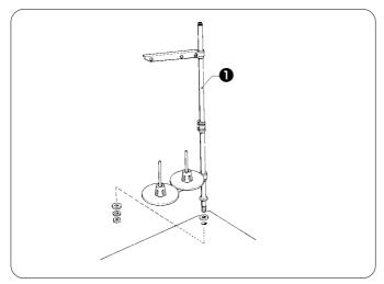
Assemble the spool stand **①** while referring to the spool stand instruction manual, and then install the spool stand **①** at the right side of the work table.
