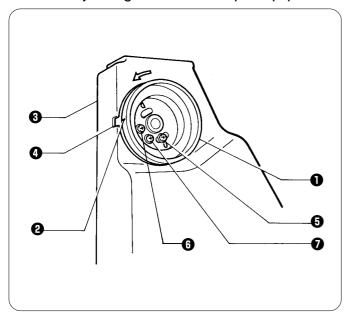
The needle up stop position is adjusted so that the index mark ② on the machine pulley ① is inside the mark ④ on the belt cover ③.
