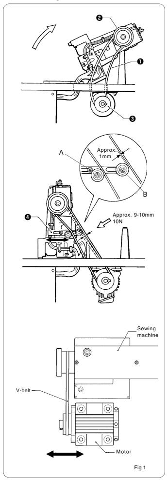
Gently tilt back the machine head, and then place the V-belt into the V grooves on the machine head pulley and the motor pulley .
