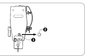
Turn the machine pulley to move the needle bar to the lowest position. Then remove the rubber plug ②, loosen the set screw ③ and then move the needle bar up or down to adjust so that the highest reference line (reference line A) is aligned with the lower edge of the needle bar bush ①.
