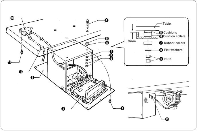
Remove the 12 screws 1, and then open the covers (panel mounting assembly 2 and main P.C. board mounting plate 3).
