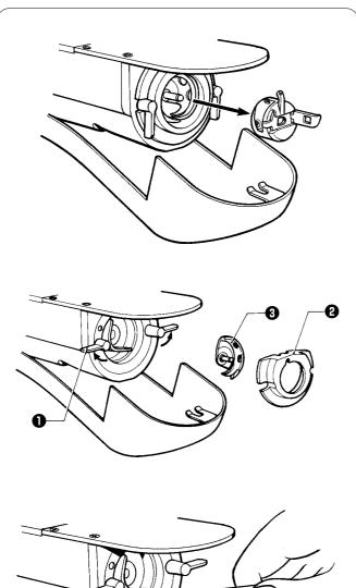
1. Pull the shuttle race cover toward you to open it, and then remove the bobbin case.
