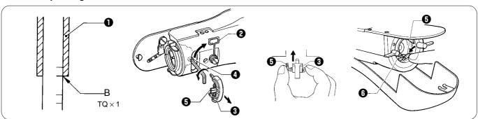
Adjust the needle bar lift amount as described below so that the tip of the rotary hook is aligned with the center of the needle when the machine pulley is turned to raise the needle bar from its lowest position until the second reference line from the top of the needle (reference line B) is aligned with the lower edge of the needle bar bush 1.
