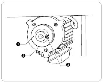
Place the motor pulley ① onto the shaft of the motor ② so that the key groove is aligned, and then tighten the set screw ③ so that the center of the V groove in the motor pulley ① is aligned as closely as possible with the center of the belt hole in the power table.
