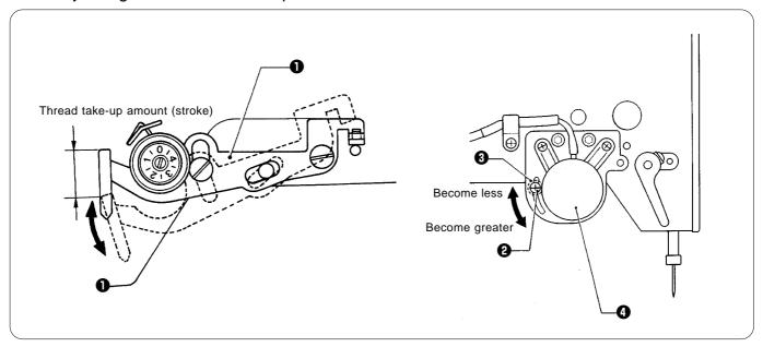
At the time of shipment from the factory, the thread take-up amount (stroke) of the thread take-up lever ① is set to the standard setting of 5 mm. You may need to adjust this setting depending on the sewing conditions to prevent the thread from pulling out at the sewing start.
