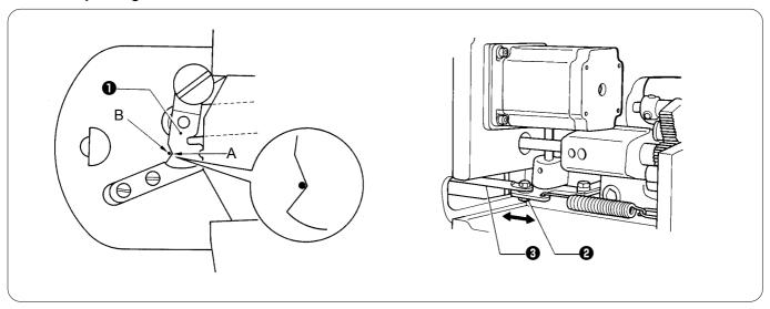
Loosen the nut ② and move the connecting rod lever ③ to the left or right to adjust so that the V section A is aligned with the index bark B on the needle plate when the sewing machine in the stopped position and the movable knife ① is moved toward the index mark.
