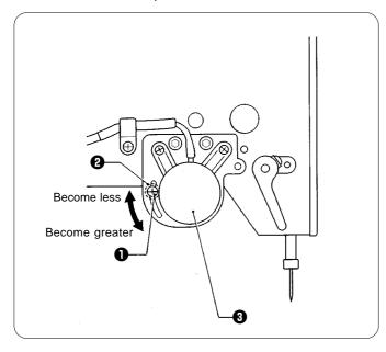
Loosen the screw 1 and move the stopper (3.57 nut) 2 to adjust the operating angle of the thread take-up solenoid 3.
