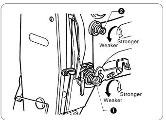
Turn the tension nut **1** (main tension) to adjust the tension as appropriate for the material being sewn. Furthermore, turn the thread nut 2(sub-tension) to adjust the remaining length of upper thread to 35 - 40 mm when the thread take-up lever is not used.
