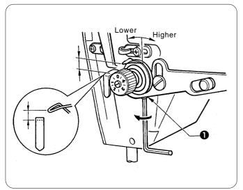
Loosen the set screw **1** and turn the tensioner body to adjust the thread take-up spring height.
