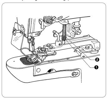
Loosen the adjusting nut **1** and turn the adjusting nut **2** to the point where it is just tight enough that the material will not slip out of place when it is slightly pulled (keep pressure as slight as possible).
