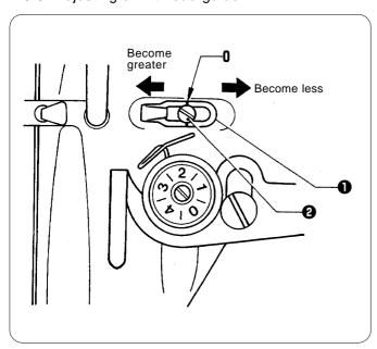
The standard position of arm thread guide R 1 is when the screw 2 is aligned with mark 0.
