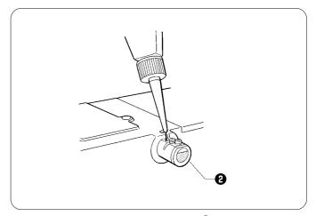
4. If using the liquid cooling tank ②, fill it with silicon oil (100 mm²/s).
