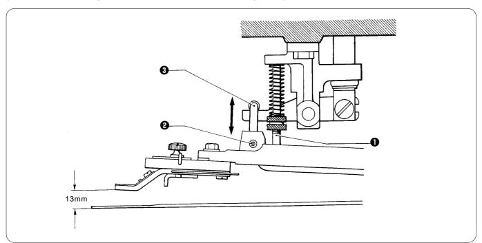
Remove the button clamp presser spring **1**, loosen the screw **2** and adjust the button clamp holder hook **3** by moving it up and down.
