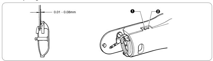
Turn the machine pulley to align the tip of the rotary hook with the needle center line. Then loosen the set screw **1** and turn the eccentric shaft **2** to adjust so that the clearance between the needle and the rotary hook is 0.01 - 0.08 mm.
