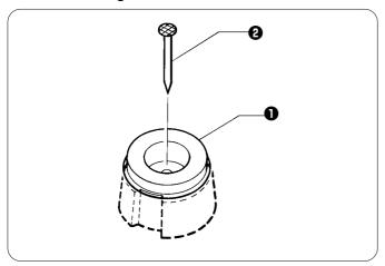
Place the two cushions ① into the holes in the work table so that the notches are aligned with the tabs in the oil pan, and secure them in place with the nails ②.
