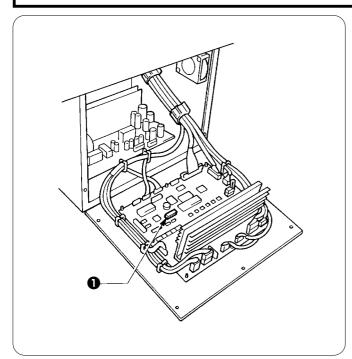
The DIP switches 1 inside the control box are used to change functions which do not often need to be changed once they have been set.
