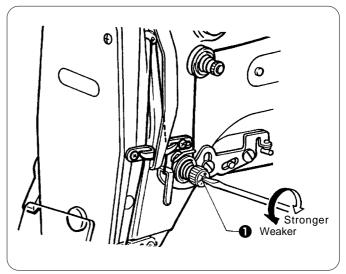
Turn the tension stud **1** with a screwdriver.
