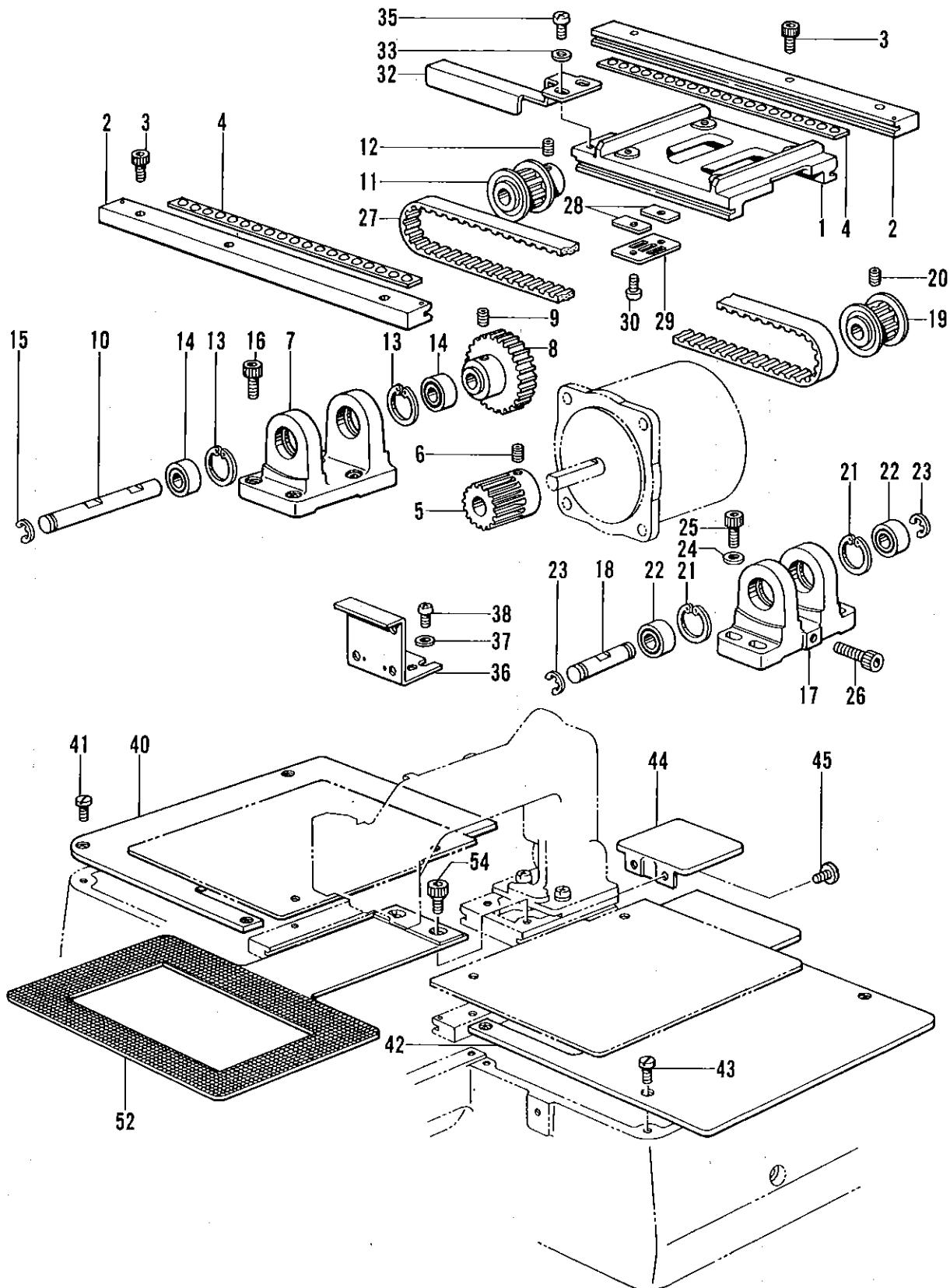
F. 駆動側・送り関係 /Feed guide mechanism/Transportführung/
