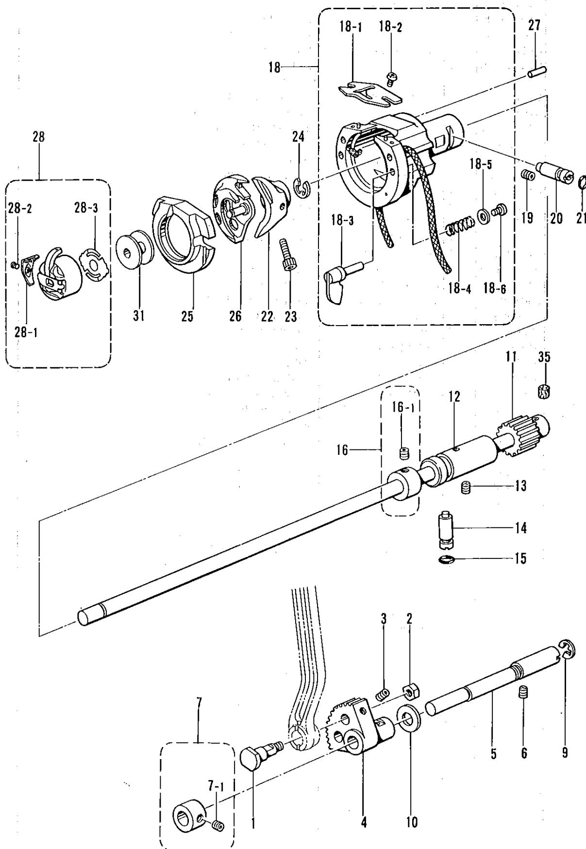
G. 下軸関係 /Lower shaft mechanism/Untere Welle/
