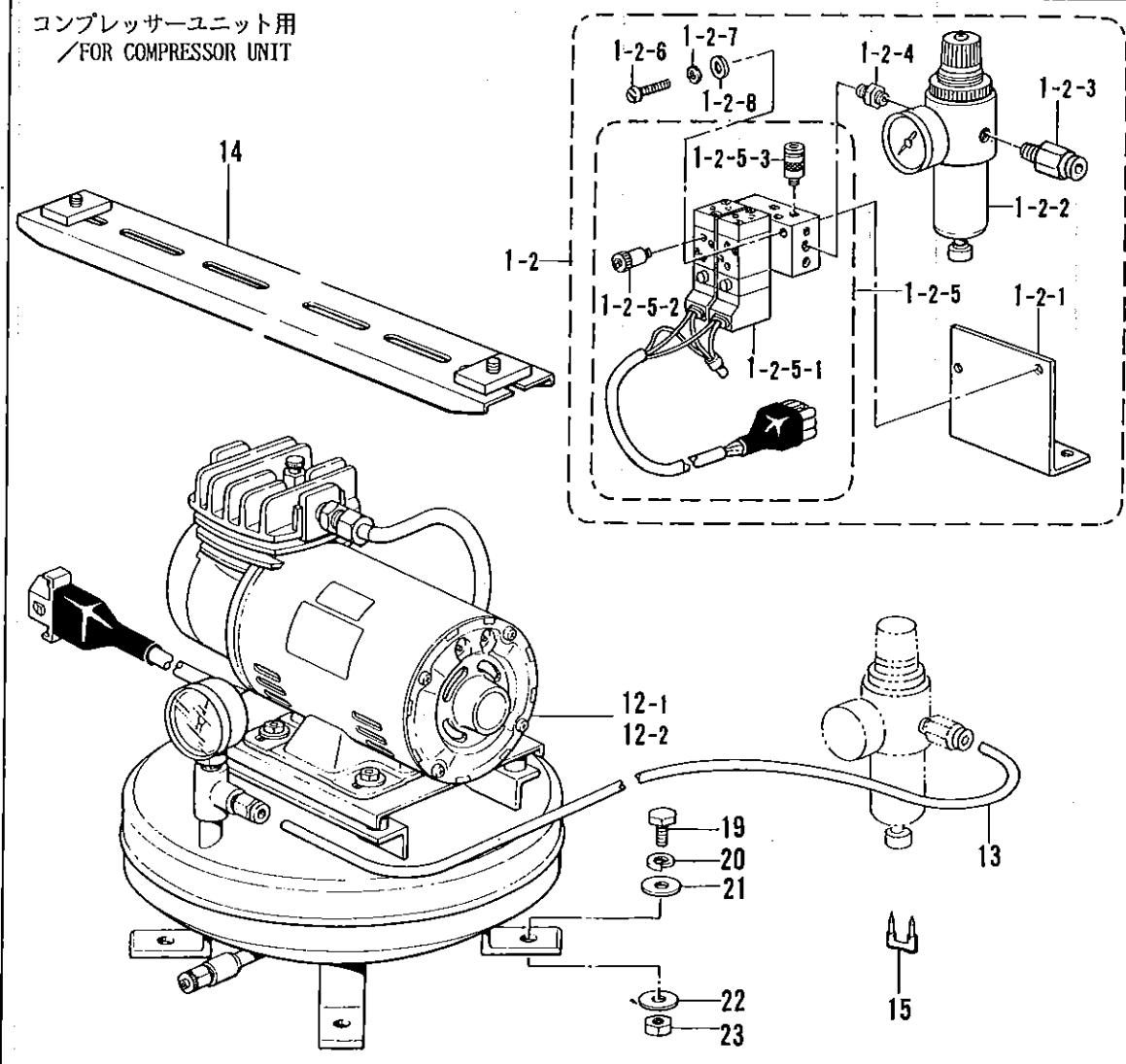
S. 空圧関係/Air pressure mechanism/Luftdruck/
