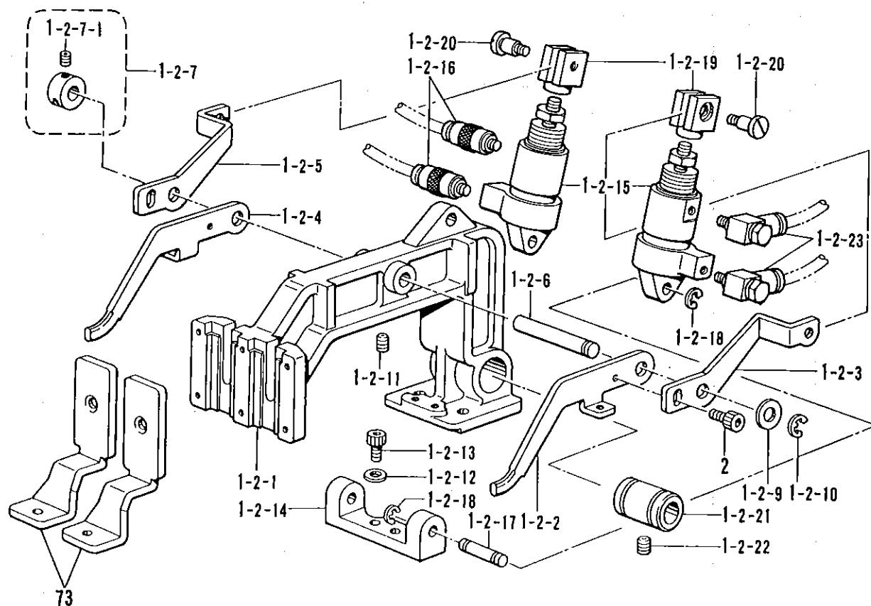
D1. 送り関係/Feed mechanism/Transportvorrichtung/
