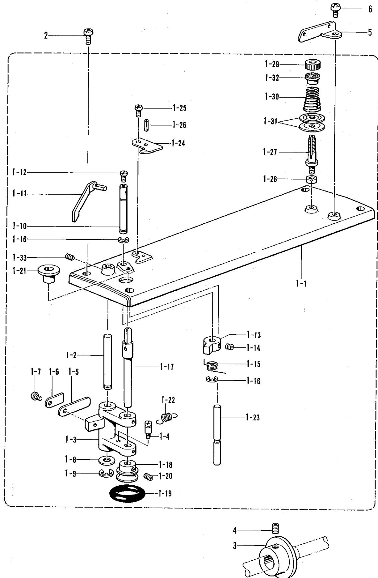
K. 糸巻関係 / Bobbin winder mechanism / Spuler /
