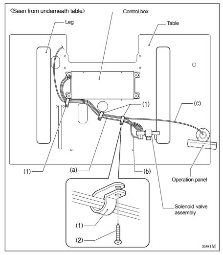
Secure the air tubes (a), the solenoid valve assembly cord (b) and the operation panel cord (c) together underneath the table with the three cord holders (1).
