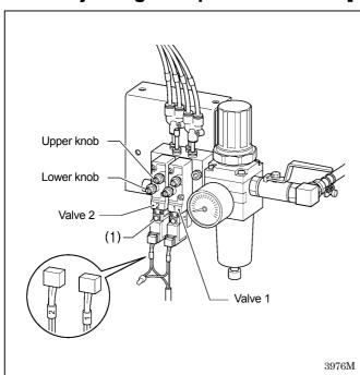
You can adjust the lifting and lowering speeds for the work clamp using the knobs on the valves.
