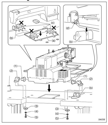
1. Place the machine head onto the table.
