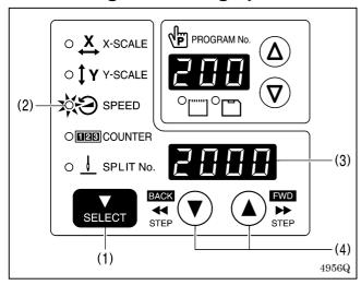
The sewing speed is set to 2000 (rpm) at the time of shipment from the factory.
