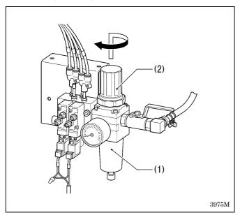
Lift up the handle (2) of the regulator (1) and then turn it to adjust the air pressure to 0.5 MPa.
