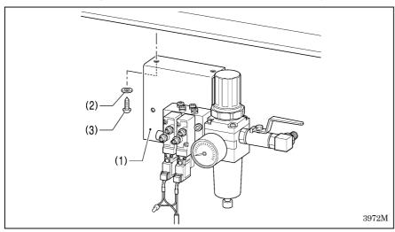
Install underneath the work table. (Refer to "3. Table processing diagram" for the installation positions.)
