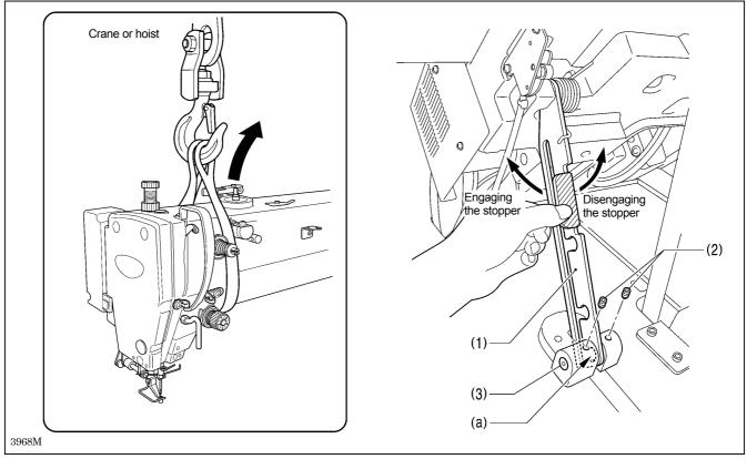
1. Tilt back the machine head, and then secure the support lever (1) at stopper position (a). (Refer to "4-5. Tilting back and returning the machine head".)
