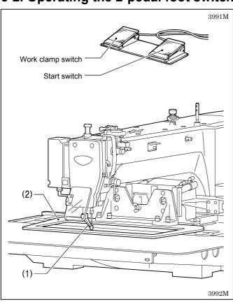
When the work clamp switch (left side) is depressed, the intermittent presser foot (1) and the work clamp (2) are lowered, and when the start switch (right side) is then depressed, the sewing machine starts operating.
