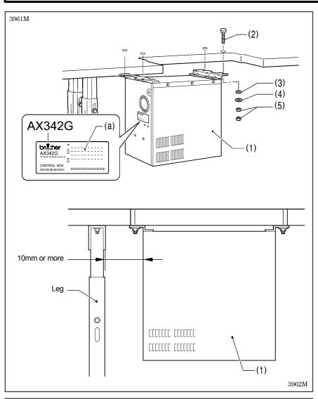
Before installing the control box (1), check that the model plate (a) on the control box (1) is "AX342G" to indicate that it is an RX-control box for BAS-342G sewing machines.
